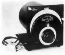
The Type 1211-A Unit Oscillator has a frequency span of 0.5Mc to 50Me which is covered in two 10-to-1 logarithmic ranges. Frequency is read directly from a 6" dial, with a slowmotion-drive dial
