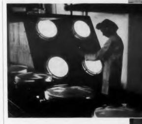
Unique photographic process, like photoengraying, uses aperture masks as negatives to print consecutively the red, green, and blue phosphor dots (250,000 of each) on CBS-Colortron screens.
