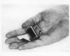
Stable tape resistors for a wide range of printed circuit applications are available either as cured, ready-to-use resistors only 1/2" long x 1/8" wide x 1/100" thick, or as uncut,
