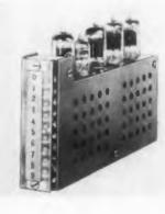
The SC-41 "Plug-In Decascale" is a direct-reading counter capable of operating at speeds up to 75,000 counts per second and resolving individual pulses separated by as little as  $5\mu$ sec. It has a five-tube decade scaling unit with a self-contained 10-light neon indicator. It contains
