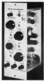
The Type 163 Pulse Generator is designed to supply rectangular pulses of less than  $0.2\mu sec$  rise time when triggered by either a positive pulse or a negative-going sawtooth from an external source. A positive pulse of calibrated continuously variable amplitude from 0 to 25v peak-to-peak, and a positive gate of 25v fixed amplitude, are supplied. The pulse and gate are identical in other characteristics.
