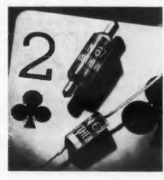
The 1N67-1N67-P is a hermetically sealed germanium diode designed for use as a 5v to 50v d-c restorer rectifier in those applications where small size, low shunt capacity, and absence of heater voltage are important. Rated for operation from -50°
