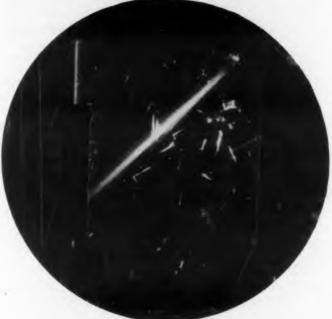
A new photographic technique has determined that the strains in commercial grade fused quartz do not prevent its use as an ultrasonic delay line. These strains are shown in the upper photo. The lower photo, made by this technique reveals no distortion if a 30 Mc/sec sound wave due to the strains.
