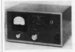
Entirely random noise with good normal or Gaussian amplitude distribution is provided by the Type 811-A Random Noise Generator. The unit is valuable for tests
