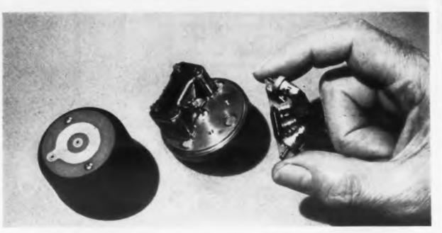
Fig. 1 (above). A disassembled preamplifier unit showing its high gain transistor amplifier. It affords improved reception, yet saves weight.
