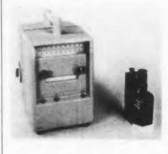
The Model 60A ruggedized galvanometer (right) and Model 61A display box (left) are designed for both field and laboratory use. The galvanometer suspension is totally immersed in liquid having a spe-
