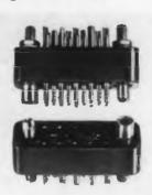
Except for the 8-contact unit, all connectors are interchangeable with similar equipment. Socket contacts are spring types which snap in and out easily without special tools. They require no "C" rings, and no undercutting is needed to seat a "C" ring on the solder-pot side. It is possible to insert insulating sleeving into insulator on the solder-pot side of both socket and pin contacts. Viking Electric, Dept. ED, 1061 Ingraham St., Los Angeles 17, Calif.
