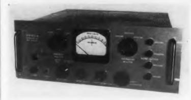
The Model RUG-1-10 makes available a random voltage source of controlled frequency spectrum and probability distribution. Examples of uses include: study of random air-load effects in airframe design, noise problems in missile guidance, study of the statistical properties of ground electromagnetic reflection, low frequency phenomena including chemical and thermal processes, and certain bioelectrical effects.
