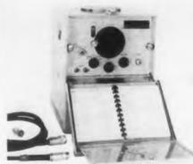
A portable frequency setting and determining instrument, the TS-175 A/U frequency meter is for general use in the 85-1000Mc range. It includes a calibration book located in the front panel,
