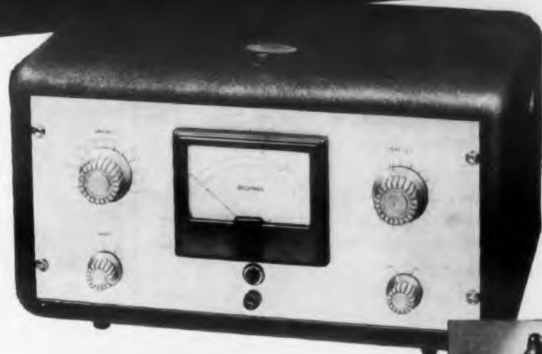
The Beckman Model V Micro-Microammeter—for the precise measurement of extremely small electrical currents. Beckman Instruments, Inc., South Pasadena, California.
