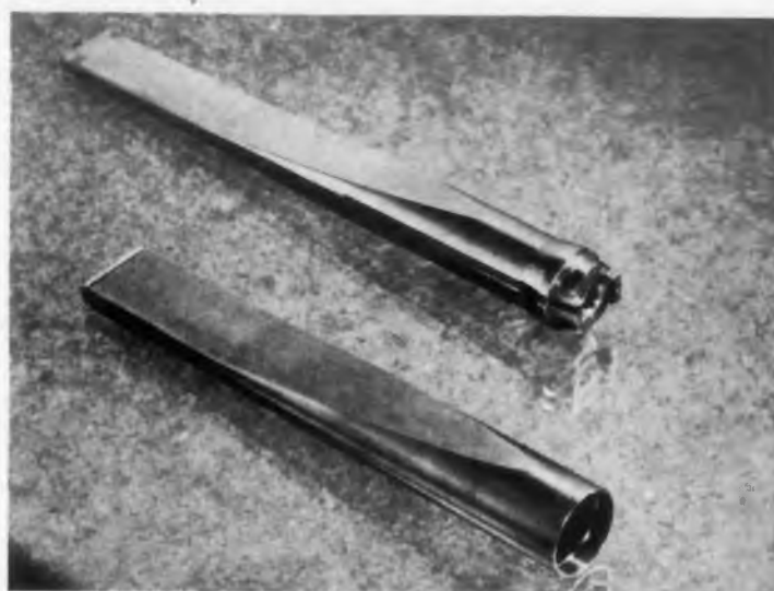
Fig. 1. A round-to-rectangular transition tube is an example of the simplest type of electroforming.
