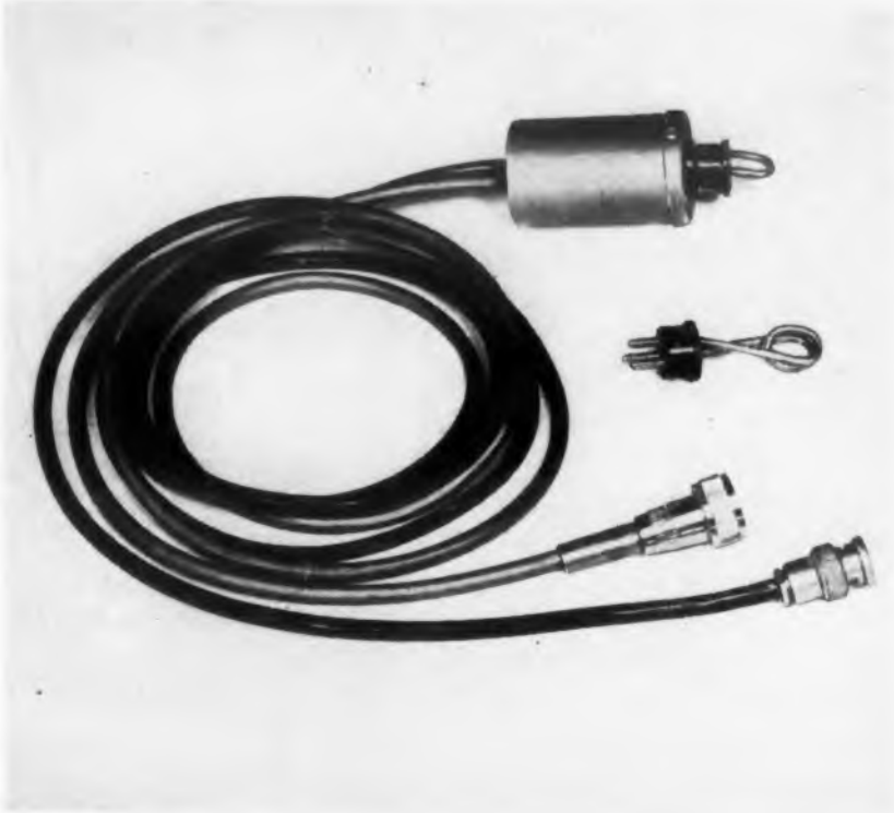
Fig. 1 (left). This resonance indicator with plug-in probes performs many of the functions of a grid-dip meter.
