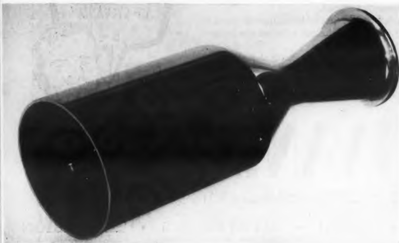
Fig. 2. Two piece taper molds, which can be screwed together (and reused), are employed to make this venturi.
