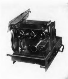
The "Cavi-Tuner''—a u-h-f tuner, has been designed as a component for TV sets to permit reception of u-h-f stations in addition to the present v-h-f channels.
