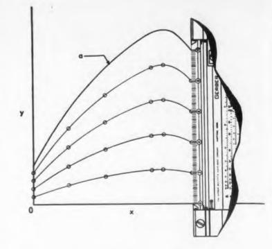
Fig. 2. The instrument in use. (Above) Here the device is being used to plot a family of curves from the single curve (a). (Below) By converting a nonlinear calibration scale (Z) to "percent values" and plotting these on the special graph paper shown at the right which is inserted into the "GraphAnalogue", the instrument then is calibrated to read corrected values directly from the original curve which might be in the form of telemetering data, oscilloscope tracings, etc.
