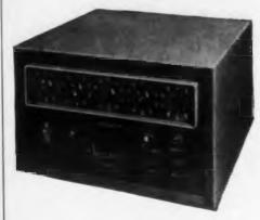
This Electronic Tachometer has been designed to measure rate, frequency, or speed by counting discrete pulses for an accurately timed interval (1sec). A clear, sharp, compact read-out is pro-
