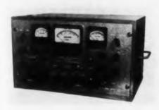
The Model TA-1 Transistor Analyzer is a current gain meter and curve tracer used to measure emitter-to-collector current gain (a) of point contact transistors,
