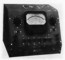
The Model TT-11 Transistor Tester provides a means of testing transistors or other semiconductor devices on a direct reading "go no-go" basis. The unit tests both junction and point-contact transistors and is not
