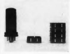
The "Perma-Memory" Multiple Scaler is a counting device permitting incoming pulses to be counted down to any desired ratio, whether the pulses are repetitive or random. Applica-
