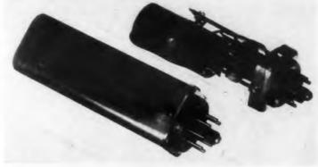
The small Rectifier-Filter circuit shown here was developed especially for reducing hum by supplying d-e heater current to the first stage of low level amplifiers. It is provided with an octal plug for convenient mounting and occupies a space above the chassis of only 1-3/8" x 1-3/8" x 4".
