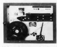
This Computer Magnetic Tape Mechanism, designed for recording and storing digital data, is a single, compact unit incorporating all the elements needed for precise,
