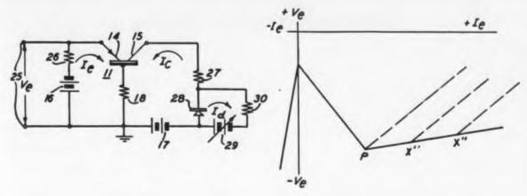
Fig. 2. Transistor Trigger circuit with current-voltage characteristics shown alongside.
