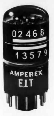
Fig. 1. The Type EIT Decade Counter Tube. A count is indicated by a rectangular luminescent spot appearing next to one of the figures 0 to 9 on the circumference of the bulb.
