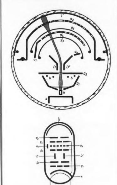
Fig. 3. Electrode structure and symbolic representation of the Type EIT Decade Counter Tube.
