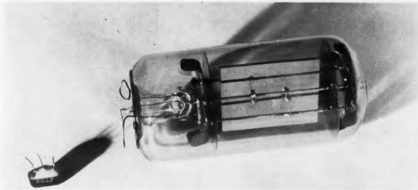
Fig. 2. Basic components of the oscillator, showing the transistor (left) and the quartz crystal unit (right).
