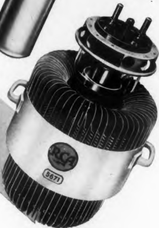
RCA-5671 SAVE—60% filament power, over comparable pure-tungsten type
