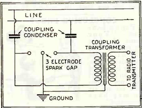
Above is the hook-up of a wired wireless system, showing how the transmitter is coupled to the line.
