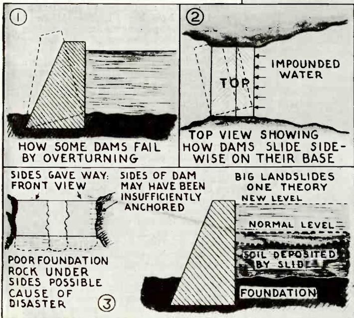
At the right of Fig. 3 above, we see how major landslides may have caused water level behind the St. Francis Dam to rise, the large deposit of silt, by its weight, increasing the total pressure on the dam. The landslide theory was advanced early by a prominent engineer familiar with the St. Francis Dam. Engineers who inspected the site of the broken dam are said to have found evidence of such landslides.
