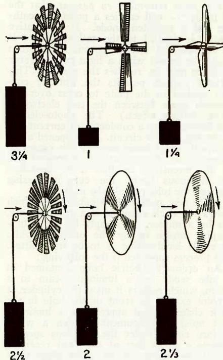
Fig. 5—The amount of wind pressure exerted on motionless (above) and moving (below) wind-wheels are indicated by black weights; left: wind-turbine; center: wind-mill; right: Venti-motor.
