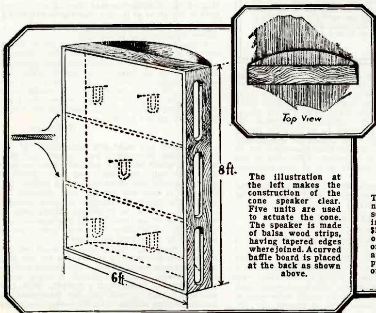
The illustration at the left makes the construction of the cone speaker clear. Five units are used to actuate the cone. The speaker is made of balsa wood strips, having tapered edges where joined. A curved baffle board is placed at the back as shown above.
