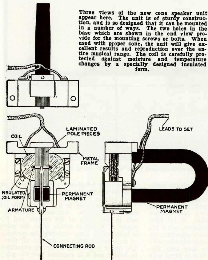
Three views of the new cone speaker unit appear here. The unit is of sturdy construction, and is so designed that it can be mounted in a number of ways. The two holes in the base which are shown in the end view provide for the mounting screws or bolts. When used with proper cone, the unit will give excellent results and reproduction over the entire musical range. The coil is carefully protected against moisture and temperature changes by a specially designed insulated form.
