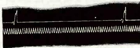
Above is a section of the paper band which passes under the two styluses, one of which is driven by an electric tuning fork at 50 beats per second. It produces the effect shown on the lower portion of the paper. The other curves on the paper are made by the synchronizing device.
