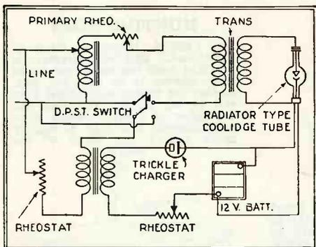
A twelve-volt storage battery with an automatic switch and relay and trickle charger, can also be used with the tube, as shown above. In this way the filament voltage is kept constant at all times.
