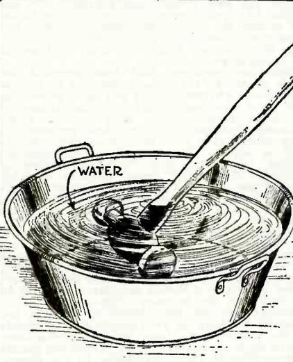
A loose hammer head, besides being an annoyance, is decidedly dangerous and should be repaired before it is used again. Such tools are generally repaired temporarily by hammering nails into the end of the handle; this method seems to be unsatisfactory in many cases. A very efficient, but little known method of tightening loose tool heads, is to soak the loose part in a pail of water overnight.—R. Wailes.
