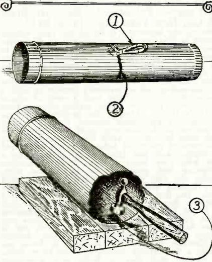
The stove pipe may be cut with an ordinary can opener, as shown in the upper illustration. The resulting ragged edge can be smoothed out with a hammer and a block of wood, as shown. Tin strips are awkward to use in contrast to this use of the can opener.
