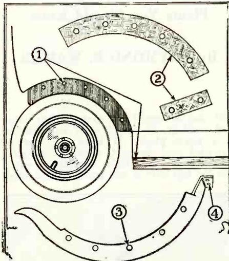
Above, 1 indicates holes to be marked on template, 2 indicates template, and 3 and 4 show holes drilled in new fender.
