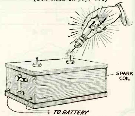
The characteristic glow of neon gas can be shown by touching one terminal of a neon lamp to a spark coil high voltage terminal.
