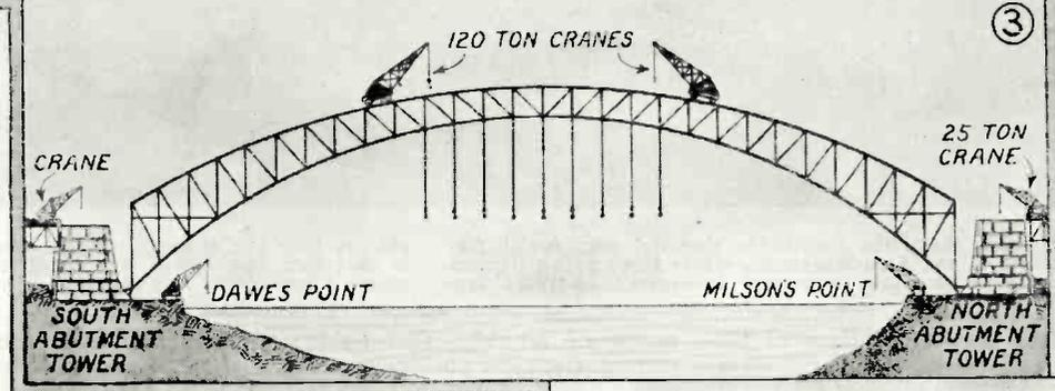
The third stage in the construction is shown at the left. After completion and final riveting, the creeper cranes start to work backwards, making way for the riveting gang.
