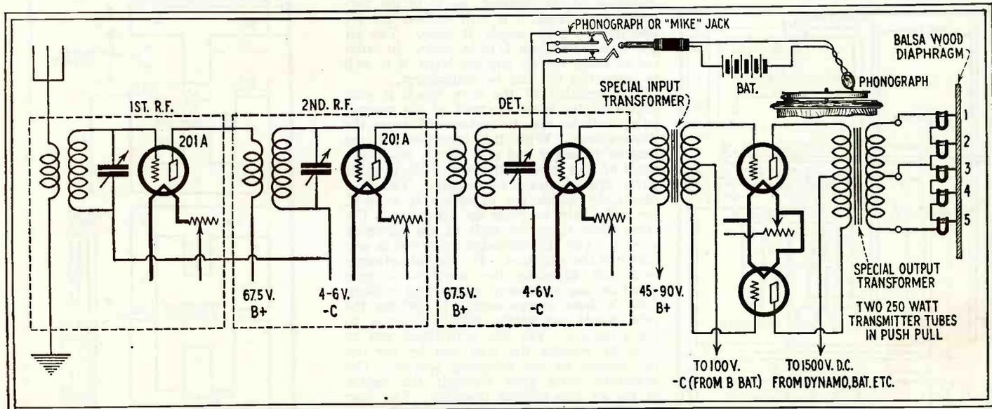
Above is the circuit diagram of the set used with the speaker described in the text for the theatre installations. Two stages of R.F. are employed.
