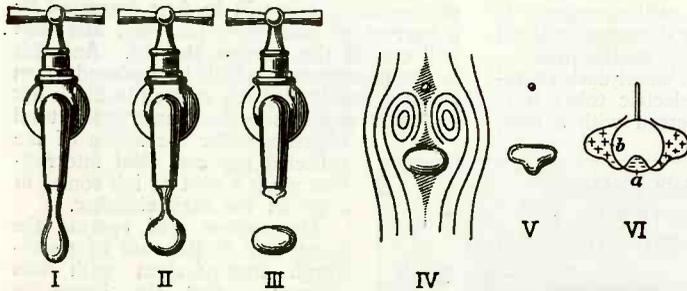
Fig. 1—The form of the falling water drop is changed materially by the resistance of the air.
