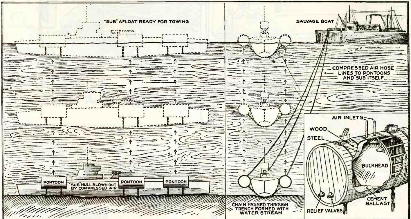
The above illustration shows how sunken submarines are now raised with pontoons by the U. S. Navy. This method was employed on the S-51 and was again used on the S-4. "Sub" hull was blown out by compressed air.
