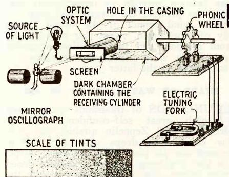
A diagram of the receiving system is shown above. An ordinary sheet of sensitized photographic paper is rolled upon the cylinder, which is placed in a dark chamber. All tints of the transmitted photograph are received in their exact value.
