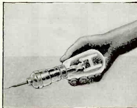
A handy tester for "live" wires made from a neon lamp.
