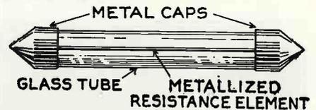
The new grid suppressor, which consists of a metallized resistance element encased in a glass tube, appears above.
