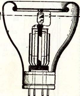
No. 1,636,921, issued to Alexander McLean Nicolson. The audion shown above, comprises an evacuated envelope, in which are placed a grid, filament, plate and a piezo-electric crystal element.
