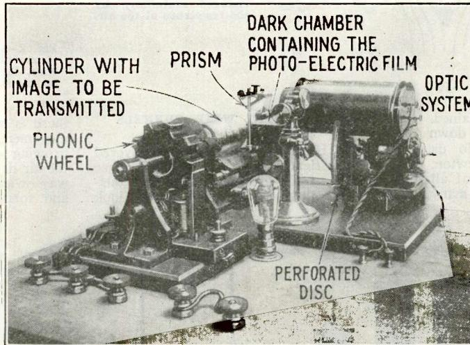
A photograph of the photo-telegraphic transmitting apparatus is shown above with the various parts marked upon the photo. The cylinder during its rotation is given a helicoidal motion. Either photographs or writings may be transmitted with this apparatus.
