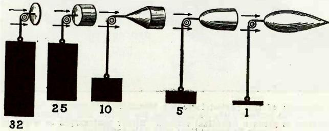
Fig. 3—Influence of the form of the body on the air resistance, which here for comparison is indicated by black weights. As we see, the resistance on the simple disc to the left, is about 32 times as great as that on the stream line Zepplin model of the same cross-section.
