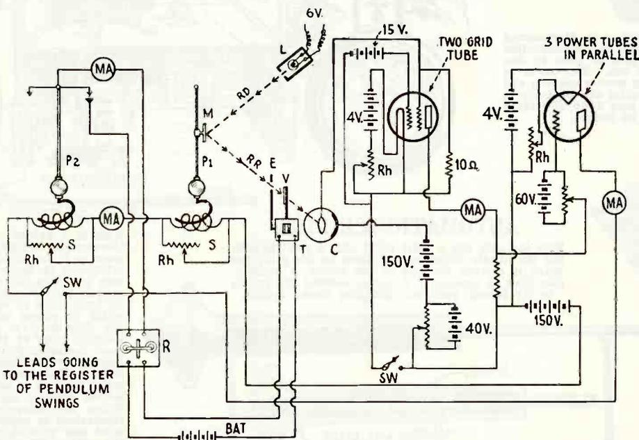
The schematic diagram of the self-regulating clock installation is given above. P1 is a free pendulum, P2 is the synchronized pendulum, SS are shunts, R is the relay, M a mirror, L the light source, and RD and RR are the beams of light. A vacuum tube having two grids is used, together with three power tubes connected in parallel.
