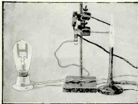
Electro-conductivity of metallic vapors is demonstrated in this experiment with a neon light.
