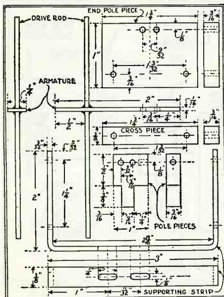
Constructional details of the supporting strip, cross piece, pole pieces, armature and drive rod are given in the above drawing. Fig. 2.
