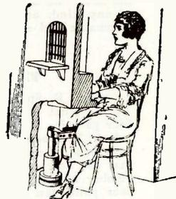
No. 1,657,459, issued to Frank Davis. This alarm system has an alarm circuit which is closed by a specially designed circuit closer. The circuit closer is worn on the leg and is operated by the other leg. A floor cord connecting the circuit closer with the alarm circuit, permits a limited amount of movement.
