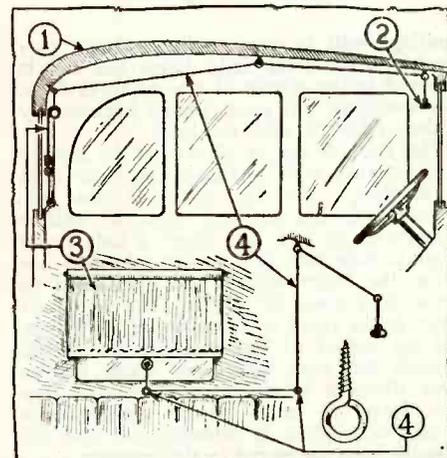
Above, 1 indicates sectional view of car, 2, knob; 3, curtain; 4, screw eyes, and linen or silk fishline.
