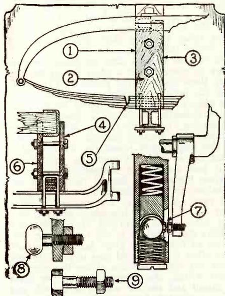
In the above illustration 1 is a blocking for a broken spring, 2, 3, 4 and 6 are boards, 5 is the broken spring, 7, broken drag link ball, and 8 a substitute for the broken ball made from 9.
