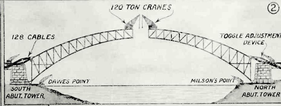
The second stage in the construction is shown at the left. The cranes have put in place panel after panel, until the span is meeting in the middle. The half arches can be adjusted as the bridge progresses by means of a nut and bolt device on the supporting cables, which may be tightened or loosened, lowering or raising the arch.
