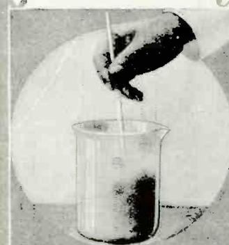
Above—making a small quantity of lead arsenate.
