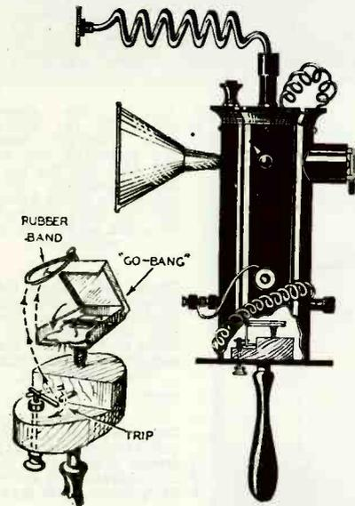
The above diagram indicates the details of the halitosis detector. The most important feature here is the "go-bang," a small metallic box provided with a trigger-like arrangement which sets off a cap when the device is released. A rubber band holds it closed until such time as the operator turns the knob connected with the trip which releases the rubber band from its catch. All other apparatus is incidental.
