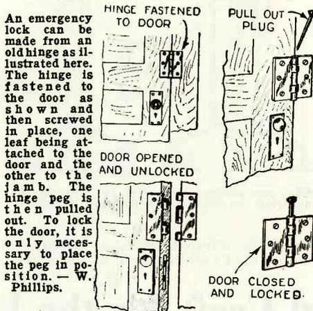
An emergency lock can be made from an old hinge as illustrated here. The hinge is fastened to the door as shown and then screwed in place, one leaf being attached to the door and the other to the jamb. The hinge peg is then pulled out. To lock the door, it is only necessary to place the peg in position.—W. Phillips.
