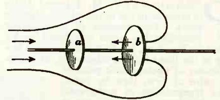
Fig. 2—A simple but surprising experiment: if one blows against the fixed disc a on the wire, the movable disc b back of it will not be blown away, but will be drawn towards a by the suction.
