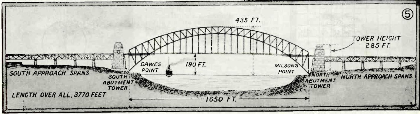
The fourth stage in the construction is shown and consists in building the road and railways. The completed bridge is shown directly above.
