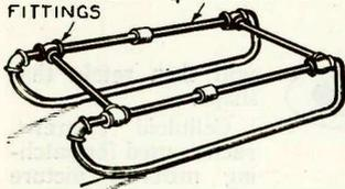
The illustration appearing here shows how a small hand sled can be made from 3/4" pipe and fittings. This can best be accomplished by filling the pipe with melted rosin or lead, and then bending it to any desired shape. Any number of cross-pieces may be arranged in order to strengthen the sled. The two runners are first bent to the desired size and then the cross-pieces of pipe are put in place.—Victor Frederick.
