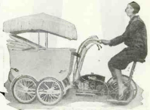
Above is a bottom view of the car which is propelled by means of pedals arranged in pairs, so as to enable two persons to drive it at the same time. The car is equipped with a light metal body and four rubber-tired wheels, similar to those used on a bicycle. Charles Mouchette and his wife invented the novelty car and are shown seated in it, in the photo at the right.
