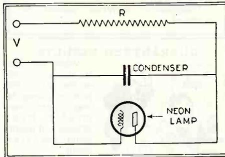
The above diagram shows how a neon lamp may be employed for measuring the capacity of condensers.
