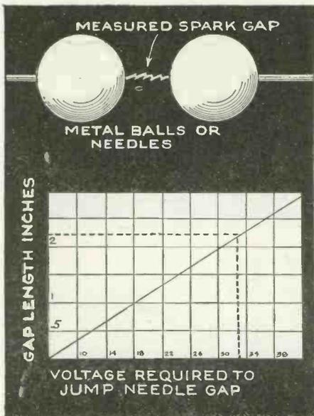
Sphere spark gaps, and in some cases needle gaps, of predetermined dimensions are used for measuring high potential discharges. When a discharge jumps a certain length of gap, the voltage is easily read from the calibration chart.
