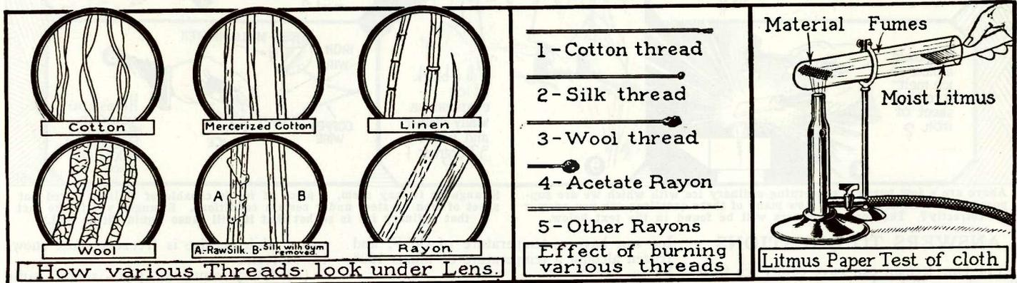
The above illustration shows how the various threads look when placed under the microscope. The effect of burning various threads and a litmus paper test of cloth are also illustrated.
