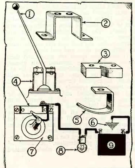
Above, 1, shift lever; 2, bracket; 3, insulation; 4, switch; 5, contact finger; 6, ground; 7, indicates a plan view; 8, the rear light; and 9, battery.
