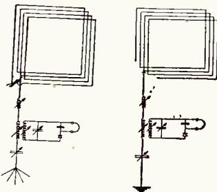
No. 1,639,913, issued to Roy A. Weagant. This aerial comprises two collecting portions which form a single antenna, one is an open loop, and the other a vertical antenna connected to the mid tap of the loop. The radio circuits are coupled to the vertical antenna. Two forms are shown above.
