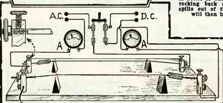
Stretch two wires over a board as shown. Connect one to an A.C. source and the other to D.C. and pass about four amperes through each. When the tension is correct the wires will vibrate. What is the cause of this phenomenon?
