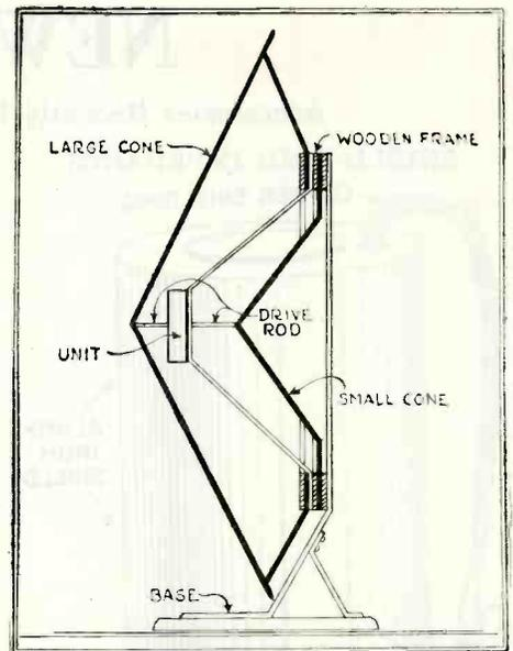
A view of the completed speaker, showing the placement of the two cones and the unit appears above. Fig. 6.
