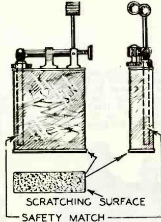
Photograph on the right shows the phoney invention cigarette lighter and at the left are the details of its construction. Note that the wick has been removed and a safety match substituted therefor. A scratching surface is shellacked to the bottom of the box. This can be obtained from an ordinary match box.
