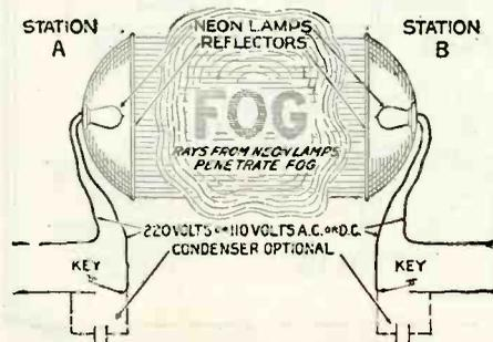
A night "blinker" set using neon lamps for signaling by dot and dash code.
