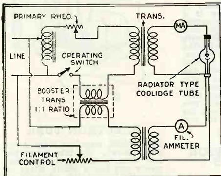
The above diagram shows a method of controlling X-ray tube filament voltage by using a booster transformer having a 1:1 ratio. This transformer has a low resistance winding in both circuits.
