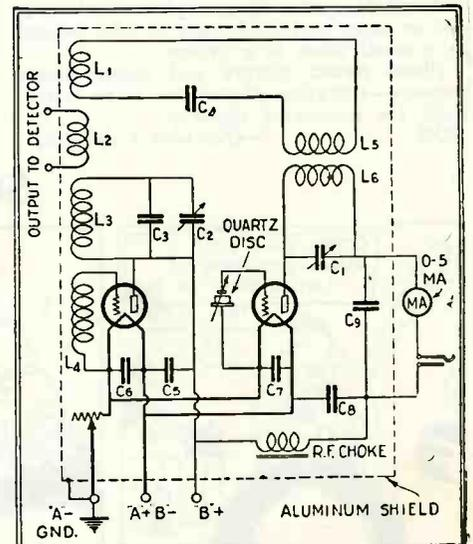
An audio frequency oscillator with quartz crystal control is shown above. A straight frequency line condenser is used for changing the frequency within the audible range.
