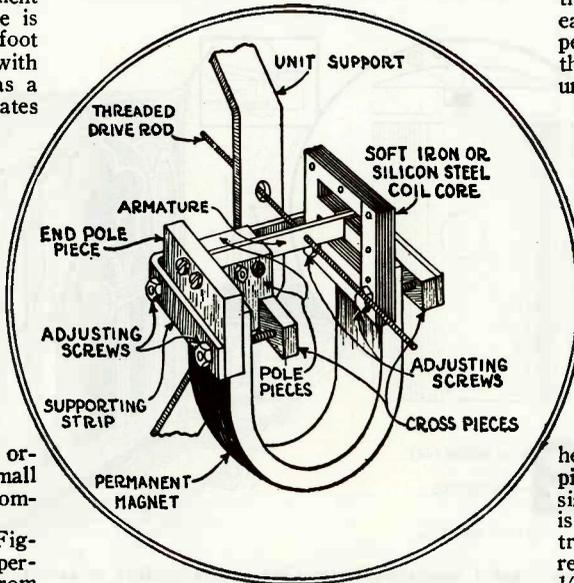
A view of the unit showing the method of assembly appears above. Note the position of the drive rod which is used to actuate both the large and small cones. Fig. 1.
