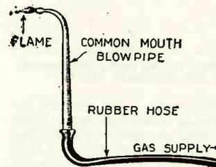
If a rubber hose from the gas supply is connected to a common blow pipe, a hot flame suitable for all blowpipe work will be obtained. The pressure obtained from the gas supply is sufficient.—Donald Manwaring.
