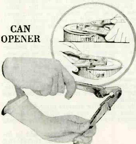
The device illustrated above and diagrammed in use is a can opener which will accommodate round or square cans. A pair of jaws on one side grip the ledge of the can. The cutter is inserted into the can and by merely opening and closing the apparatus, the cutter can be made to slice off the entire top and turn down any sharp edge which may be formed.
