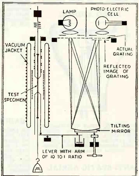
The mechanism used to measure one-billionth of an inch is shown above.
