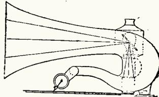
No. 1,658,030, issued to Fred Adams. This picture exhibitor for disc record talking machines has a slip disc slotted to expose sound grooves and provided with a marginal row of pictures. A baloptican picture projector is carried by the tone arm. The pictures are thus exhibited in synchronism with the sound reproductions.
