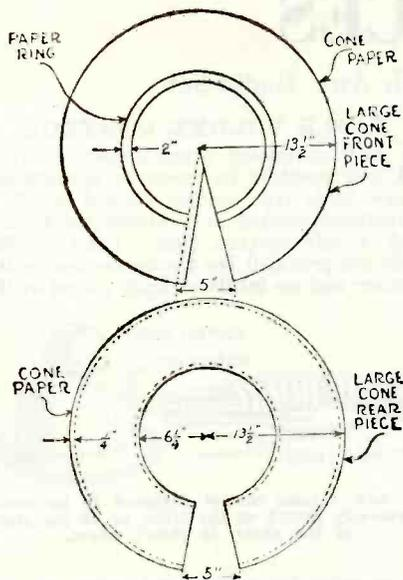
Both the front and back faces for the large cone are shown above. A paper ring 2 in. in diameter is glued on the front of the cone as shown. Fig. 4.
