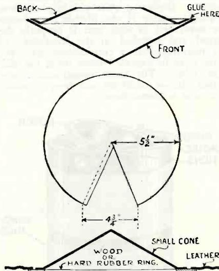
The uppermost illustration shows the method of gluing together the large cone, the next gives details of the smaller cone, and the last one shows how this cone is mounted. Fig. 5.
