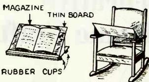
A simple magazine rack can be constructed as shown here. It is made of plywood and is very light. Four small rubber cups fastened to the base hold it on the arms of the chair without slipping. This rack can be made in various sizes, in order to fit the individual requirements.—C. R. Van. Reporter No. 16,643.
