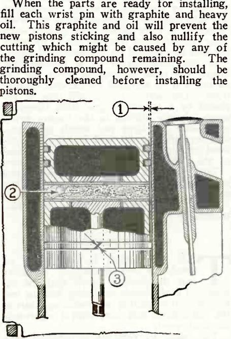
Above 1 shows .002-inch piston clearance; 2, wrist pin hole filled with graphite and oil; and 3, a clearance of .01 inch at joints of piston rings.
