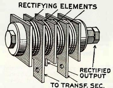
Above is a view of the dry rectifying element of the full-wave type.
