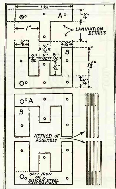
Lamination details and the method of assembly are given above. Either soft iron or silicon steel may be used. Fig. 3.
