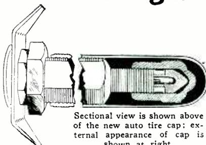
Sectional view is shown above of the new auto tire cap; external appearance of cap is shown at right.
