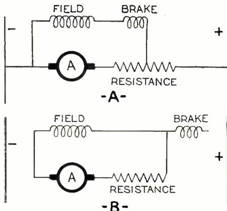
Q. 2109. Circuit diagram for dynamic braking system for electric motors.
