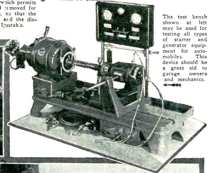
The test bench shown at left may be used for testing all types of starter and generator equipment for automobiles. This device should be a great aid to garage owners and mechanics.
