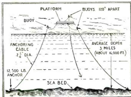
Method of anchoring seadrome, utilizing stranded steel cables 2 1/4 inches in diameter.
