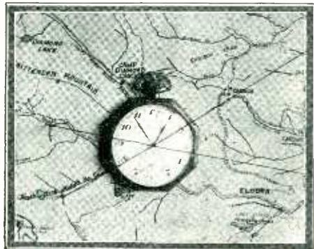
A number of practical uses can be found for your watch if you remember that each minute division on the dial represents an arc of 6 degrees. Its use as a protractor and direction indicator is shown by the photograph above. The arc between each two consecutive numbers equals 30°.—H. E. Benson.
