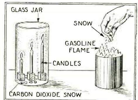
Extinguishing candles with the snow and putting out a gasoline flame with it.
