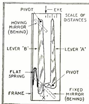
The drawing to the left shows the series of levers which operate the mirror in the range finding device. The scale of distances may be easily seen in the photograph to the right and the relative positions of the rest of the mechanism located.
