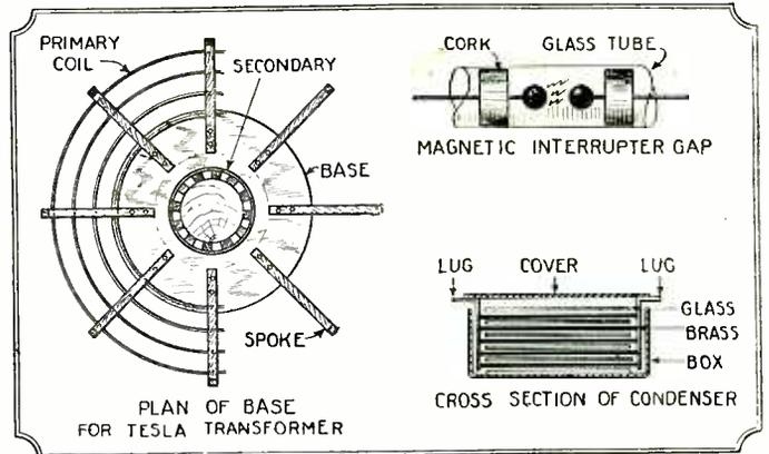
Here is shown a cross-section of the Tesla coil with the plan of the base. A magnetic interrupter gap is shown also and the cross-section of the very substantial condenser required for this apparatus.
