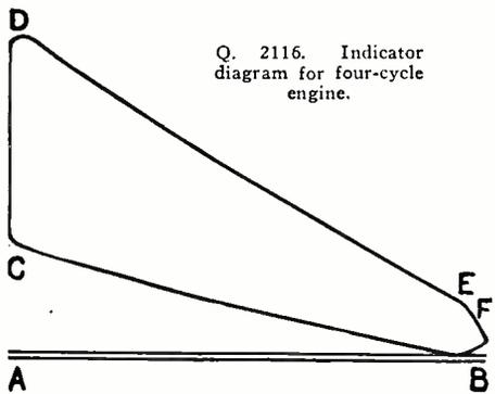
Q. 2116. Indicator diagram for four-cycle engine.
