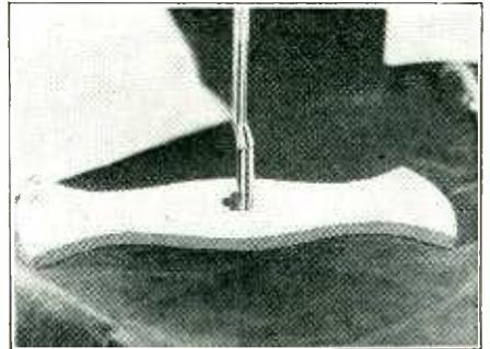
The two small screw holes and one  $\frac{3}{4}$ " hole to pass the center dowel stick are next drilled in the lower end piece. The center hole should be only slightly larger than the dowel.
