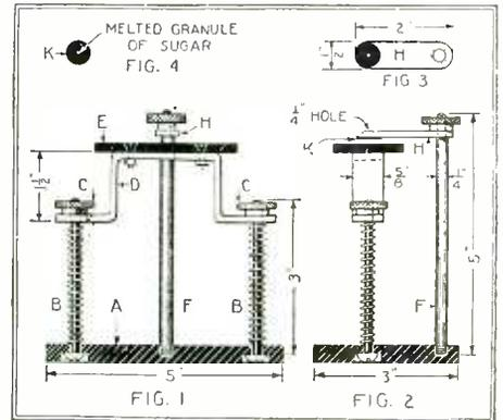
A magnification of 300 diameters may be obtained by the use of a melted sugar lens in the small microscope above. High illumination is necessary because of the very small size of the lens.—E. L. Richardson.
