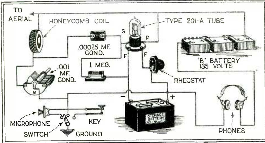
Q. 495. Picture diagram of a combination low power transmitter and receiver with three-way change-over switch for receiving, phone transmission and key. The circuit used in this set is the well known Colpitts.
