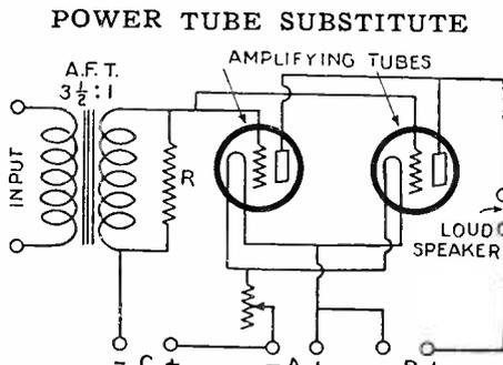
The cone type of loud speaker, being very sensitive to noises of all kinds, is operated most successfully in conjunction with non-distorting power tube amplifiers. Power tubes being more expensive than the ordinary amplifying tubes, two tubes of the latter variety may be connected in parallel, and thus deliver an undistorted output.
