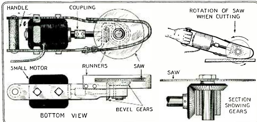
The diagram at the left shows how a motor-driven circular saw can be easily constructed. Great care should be taken to see to it that the saw runs in the direction of the arrows, because in this way it will cut down into the wood; whereas if it rotated in the opposite direction it might run away from the work.
