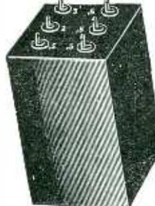
This is the high capacity 500-volt tested condenser system used in the standard "B" Battery Eliminators. Contains 4 condensers, all in one housing, as follows: 4 mfd., 2-mfd., 1/2-mfd., 1/2-mfd., total 7 1/2-mfd. Complete as illustrated, with 5 terminals; in enameled tin shell.
