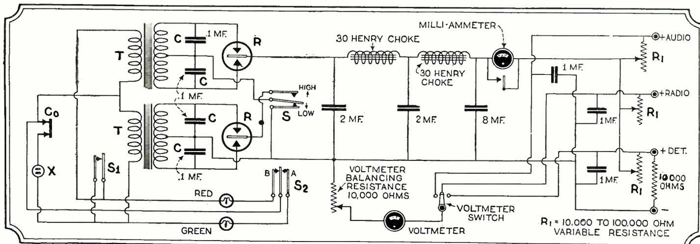
In the diagram above, notice the compound switch, S, S1, S2, for change-over from low to high voltage. The voltage control resistances, R1, are an interesting feature and permit fine variation of output. Although 30
