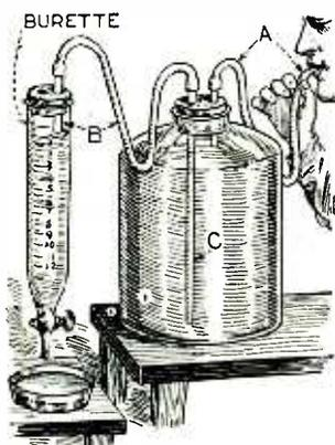
Blow in tube A until solution is above zero mark in the burette. Lower end of tube B is even with zero mark. Excess solution siphons back automatically into the stock jar. Tube C must always be partially submerged. — David N. Roush, Rep. No. 1017.
