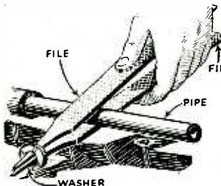
An efficient wrench for turning pipes may be improvised by fastening the handles of two flat files with a washer as shown. — H. W. Hepler.
