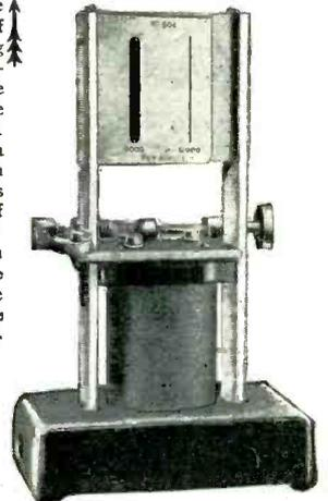
The vibrating apertures of the speed-counter may be easily seen in the above photo. The thumb screw at right is used to adjust vibrator armature.
