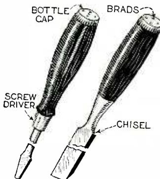
Old crown cap bottle tops may be braded to the handles of carpenter's tools to prevent the handle being split by hammering. Smooth down sharp edges to prevent cutting hands. — Wilson G. Walters, Rep. No. 6385.
