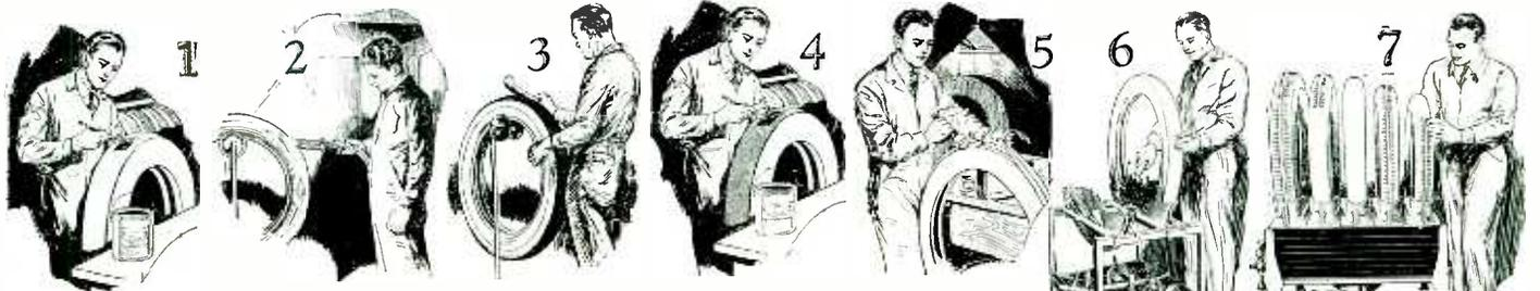
Successive stages in retreading tires: 1—Old tire painted with a special liquid and 2, heated with torch flame. 3—Charred rubber is scraped off, rubber being devulcanized. 4—Vulcanizing liquid applied, and at 5, new rubber is put on tire. Tire is put in mold, 6, and cured at 7.
