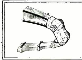
No. 1,574,898 issued to Jason A. H. Johnson. This invention relates to a cover for spring shackles on automobiles. It consists of a boot of leather or similar material, which is laced about the spring ends and shackle bolts and protects the moving parts of the spring assembly from the intrusion of injurious dust and grit. A cover applied in this fashion also functions to prevent the leakage of grease from the spring leaves.
