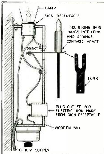
light will light up. If the iron is wanted in a hurry it is removed from the hook, cutting off the light, and laid on some non-combustible object on the bench. As the work progresses the iron is hung on the hook when not actually in use which automatically connects the lamp in series with it. Thus while not in actual use the current through the iron is reduced to such a value as to just keep it hot without overheating
