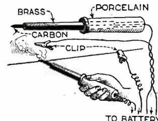
Carbon-tipped brass rod inserted into porcelain insulator makes efficient 6 volt contact soldering iron. — W. Codder.
