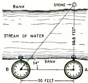
With the aid of an elementary knowledge of trigonometry, the figures on a watch dial may be used to find out the distance across a stream. The Pythagorean hypothesis ( $BC^2 = AC^2 + AB^2$ ) is used here.—Charles Rugler
