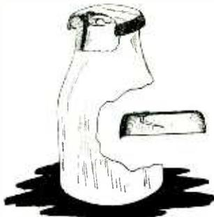
No. 1,575,319 issued to Ryk Cruyff. This invention consists of a cap of aluminum or other light metal which, when fitted over the top of an unopened milk bottle, bears a cutting blade which punctures the paper cap and on being turned, cuts it away. The aluminum cap may be used as a cover for the contents after the bottle has been opened.
