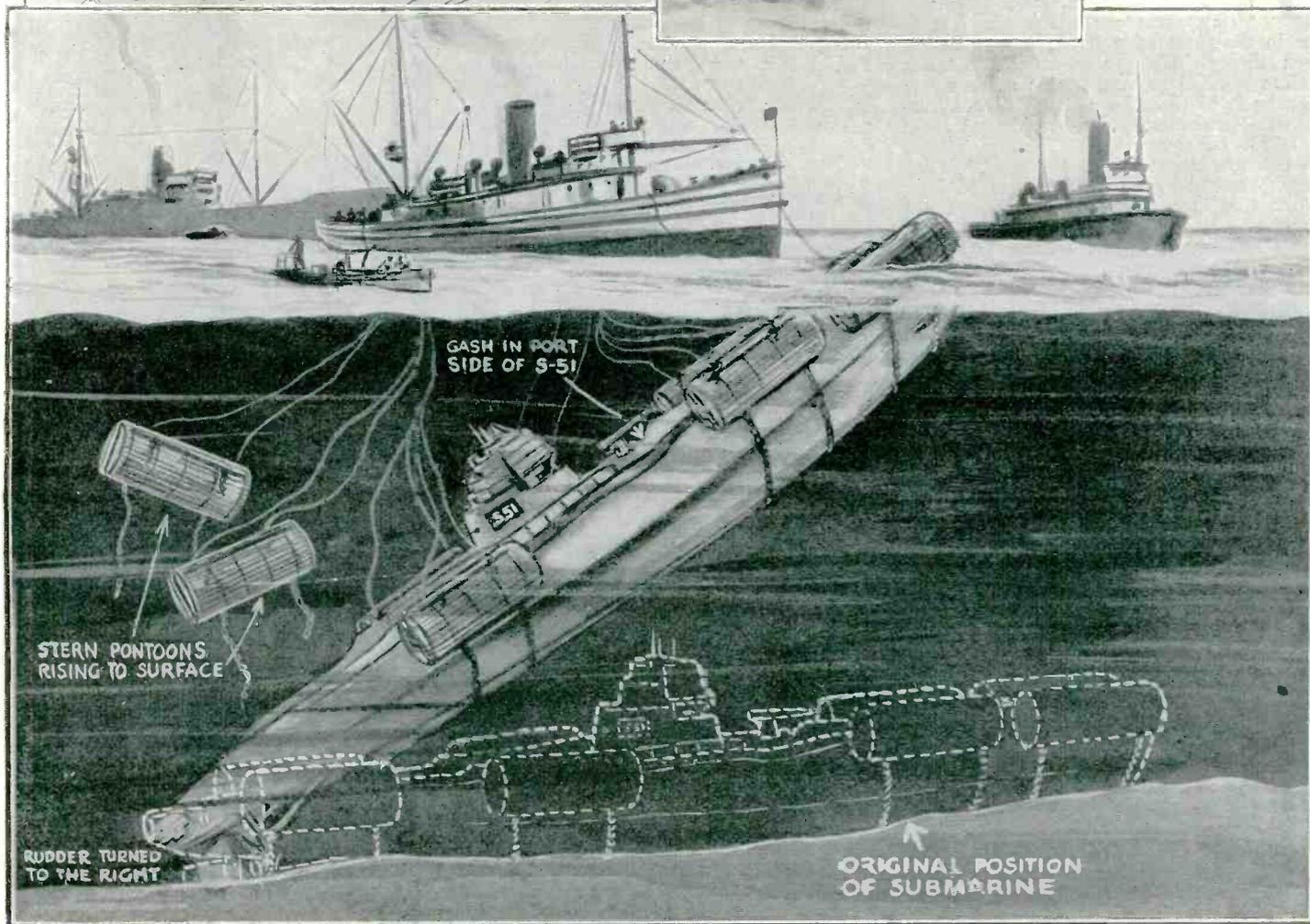
The drawing above illustrates the method of placing the pontoons so that they would exert the greatest possible lifting power on the wreck. Commander Ellsberg decided, after the rear pontoons had broken away and barely missed a surf-boat in rising, that the sub should be lowered again.
