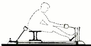
No. 1,577,809 issued to Edward T. Randall. This apparatus incorporates many of the features found in expensive gymnasium equipment. A sliding seat permits its use as a rowing machine, and means are provided for the use of coil spring exercisers and Whitley cable exercisers.
