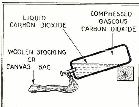
Getting ready to make carbon dioxide snow. Note bag into which gas is to flow.
