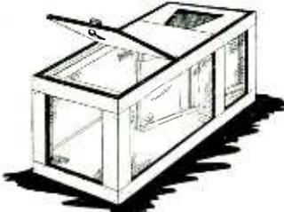
No. 1,578,061 issued to Jacques Abadie. This trap utilizes the knowledge that a roach prefers an opening only slightly larger than his body to one much larger. The bait is placed in a screened, covered box which is entered through a wedge-shaped passageway containing slots of various widths. The roach, attracted by the bait, chooses the slot most suitable to its size, enters the box and is unable to find the way out.
