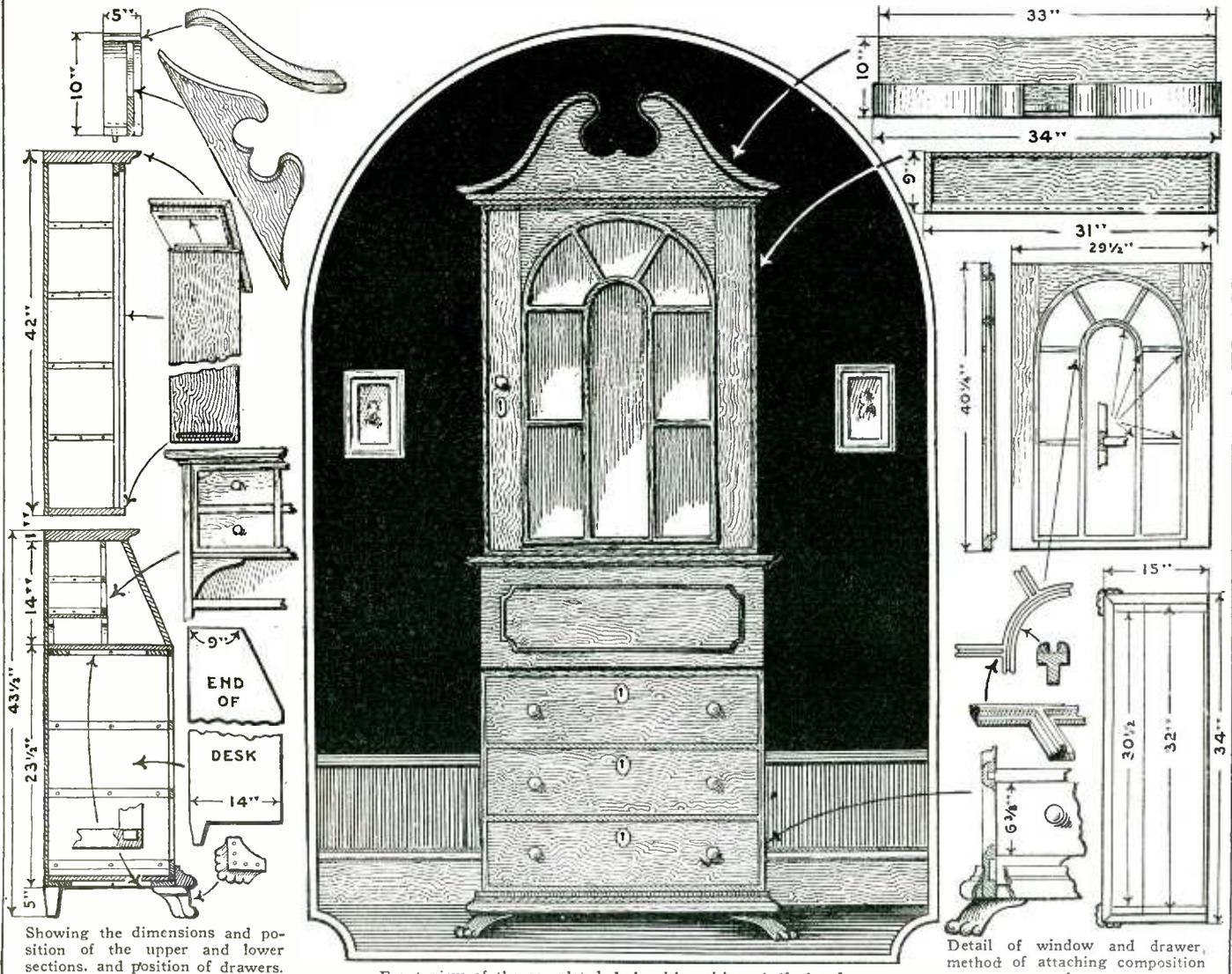
Showing the dimensions and position of the upper and lower sections, and position of drawers.
