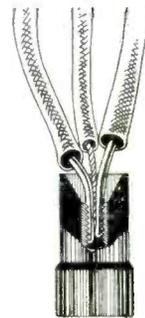
For joining two or more pieces of wire together without soldering the wires these nuts are very convenient. The ends of the wire are bared and pushed into the nut which cuts its own thread on the wire and makes a permanent connection. It is not necessary to tape the joint and four or more wires may be joined together with one nut.—Tork Company.
