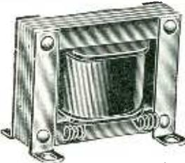
This excellent choke, especially manufactured for "B" battery eliminators, and used in the standard eliminators, has about 40-millihenry capacity, (10,000 turns of No. 32 wire) and is warranted to do the work right. Will not heat or burn out under normal load.
