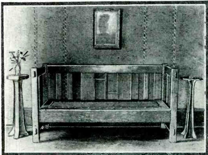
A VERY simple and dignified settee that can easily be used to grace any room in the house is illustrated in the photograph at the immediate left and is shown in detail in the reproduced drawings directly above. Note how simple each and every part is made. Plain mortise and tenon joints are used throughout and the parts are glued or pinned in place. The following material is required:
