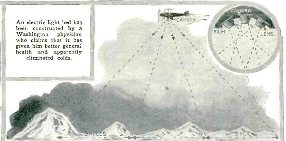
Three cameras of a new type have been assigned to the Alaskan Mapping Expedition for an extended aerial survey. From a height of 15,000 feet an area of 9 miles of territory may be mapped at one exposure.
