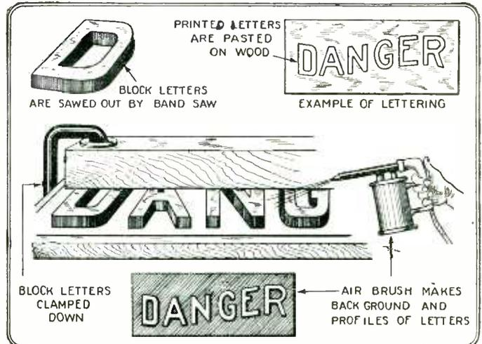
Printed letters are pasted on wood. Block letters are sawed out by band saw. Example of lettering. Block letters clamped down. Air brush makes background and profiles of letters.
