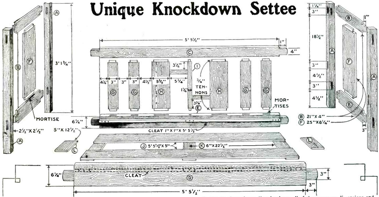
In the drawings shown directly above, all of the necessary dimensions and details for the construction of this unusual and handsome settee are shown. The carpentry work required is very simple and can be performed by anyone who is at all handy with ordinary woodworking tools. There is no undesirable complication.
