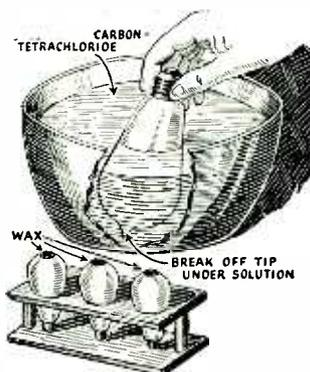
Old electric light bulbs filled by breaking off the tips in a bowl of carbon tetrachloride, make very effective fire extinguishers for home use. Breaking off bulb in flame releases chlorine which puts out the fire. — Dorothy J. Newbury.
