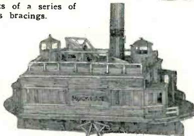
SEVENTH PRIZE—\$15.00 was the award decided on for the ferryboat "Rockland" built by Warren C. Brown of Ossining, New York. The paddle wheels can be made to rotate, which motion is transmitted by means of levers to the beam on top of the ferry. There are two drive ways, one on either side of the engine-room.
