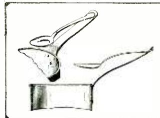
No. 1,580,582 issued to Alvin E. Carman. A simple slot cut in the end of the handle of a kitchen utensil acts as a receptacle for the handle of a mixing spoon and keeps the spoon out of the way of the utensil cover and prevents its becoming overheated.
