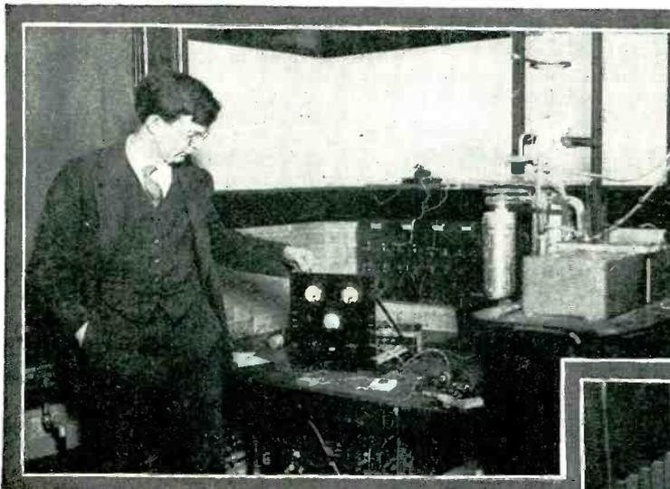
HERE is the latest apparatus developed by the Bureau of Standards for counting electrons. The process utilizes high frequency apparatus similar to that familiar to radio fans. L. F. Cutiss, expert on gamma rays at the Bureau of Standards, is standing in front of the control board. Scientists have been experimenting for years with various theoretical methods of counting electrons, but until now the apparatus has been very complicated and the results all too uncertain.
