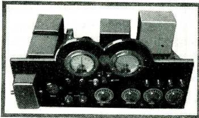
At left is a top view of the "B" eliminator which shows the positions on the condenser bank, transformer, chokes, and Raytheon tube sockets. Above may be seen the panel arrangement with meters and controls.
