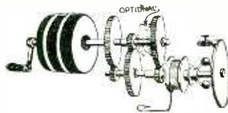
Motor is shown at left. Any sort of trigger release may be attached to the governor brake.—R. J. McHale.
