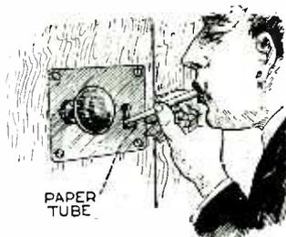
Graphite powder made from pencil leads if blown as shown, into a door lock, will lubricate it thoroughly. — Wendell Rich.
