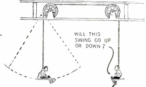
Two swings are supported at the opposite ends of a rope which passes over two freely rotating pulleys as indicated in the diagram. If two boys of equal weight are seated in the swings, what would be the effect on the positions of the swings, if one of the boys should set his swing in motion?
