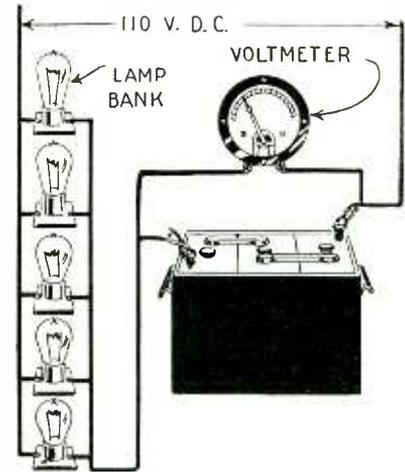
A voltmeter is shunted across a 6-volt storage battery which is connected to a 110-volt D.C. line. A lamp bank having 20 ohms resistance is connected in series with the battery. If the voltmeter will read only up to 7 volts, can it be used in this circuit? Could it be used on a 220-volt line?
