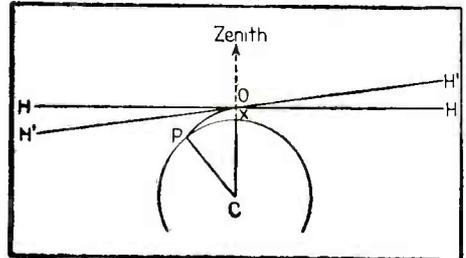
The Dip of the Sea Horizon: X Is the Height of the Observer, in Feet, Above Sea-Level. HH' is the True Horizon of the Observer at O, Which Is at Right Angles to the Direction of the Plumb-Line. PO Is the Path of the Line of Sight to an Object, P, the Most Distant Point on the Earth's Surface Visible from O; the Line is Curved on Account of Refraction, Which Is Greatest at Sea-Level. The Observer at O Sees P in the Direction OH', Owing to the Effects of Refraction.
