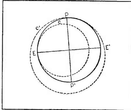
Diagrams Illustrating Why a Degree of Latitude on the Earth Is Shorter at the Equator Than It Is at the Poles.
