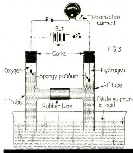
Fig. 3. With This Simple H Tube and Spongy Platinum Taken from an Automatic Gas Lighter, the Polarization Current or Reverse Current Can Be Measured.
