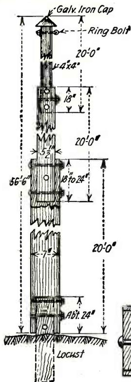
pole is made with  $\frac{3}{4}$  inch boards cut to the proper width. The top piece is solid, 4 inches by 4 inches tapered down to about 3 inches at the very peak. Each connecting section is bolted together with three wagon bolts.
