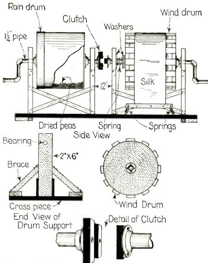
The Combination Rain and Wind Machine for Amateur Stage Productions, Illustrated Above, Is Simple to Build and Can Be Made in Different Sizes According to the Dimensions of the Stage, and the Show Itself. The Small Model of This Machine Proves Very Useful in Staging Miniature Productions With Marionettes or Dolls.
