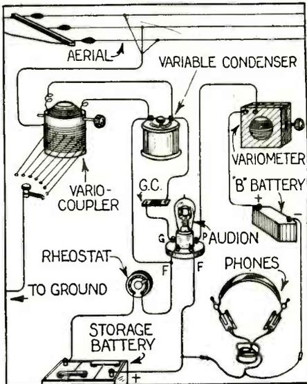
A Simple Form of Short Wave Regenerative Tuner Is Shown Herewith, Employing a Single Variometer to Tune the Plate Circuit.
