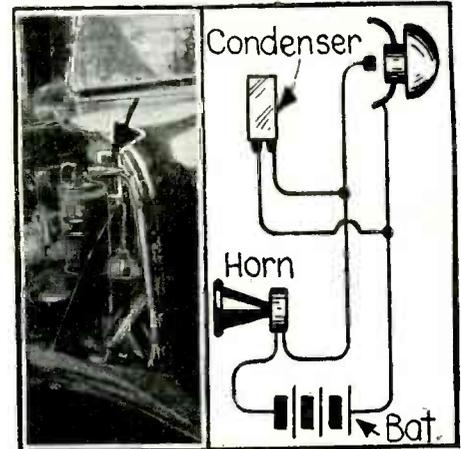
A Telephone Condenser Shunted Across the Horn Button Wires Saves Burning the Contacts.
