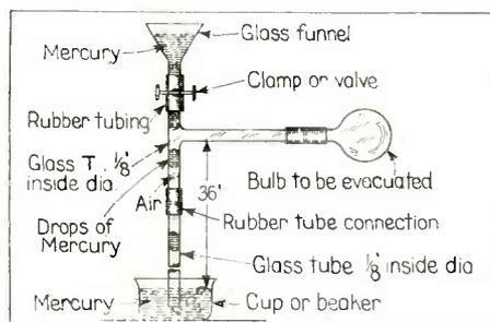
The Diagram Above Shows How a Simple Mercury Vacuum Pump of the Sprengel Type Can Be Constructed by the Experimenter.
