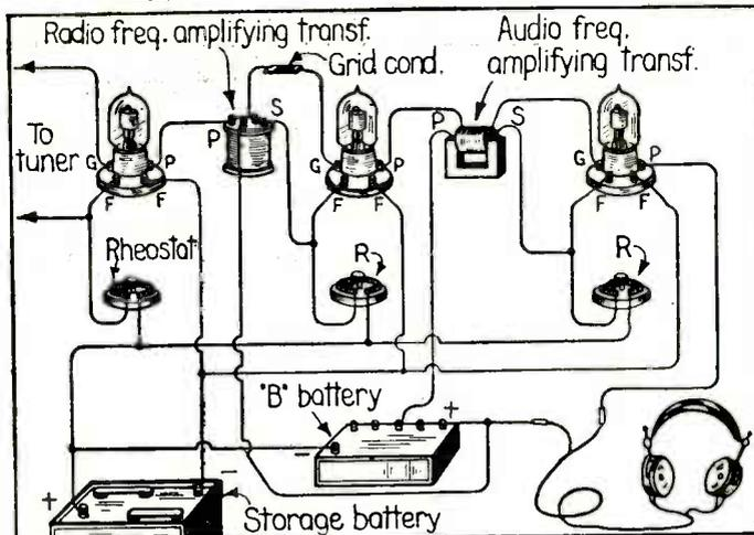
This Circuit Gives the Connections Necessary for One Step of Radio-Frequency Amplification, a Detector and One Step of Audio-Frequency Amplification Using Common A and B Batteries. The B Battery Should Have a Voltage of 40 to 60 Volts With a Tap at 22½ Volts.
