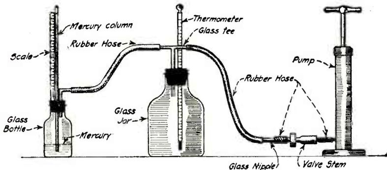
An old valve stem is sawed off near its base and filed off so it will fit tight in the rubber hose that is attached to the pump. The valve stem must be placed in a reverse position. The coil spring is removed from the valve inside the pump, so the valve can work freely. In some automobile pumps reversing the rubber washer will serve the purpose, in others simply soldering a piece of tubing to the air vent is more satisfactory.
