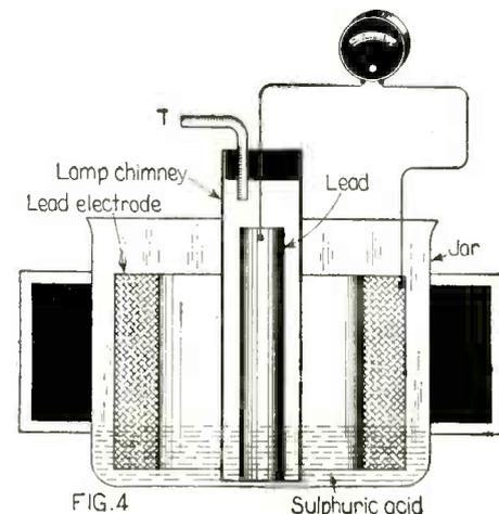
Fig. 4. A Simple Gas Battery. Illuminating Gas Is Led Through the Tube T.
