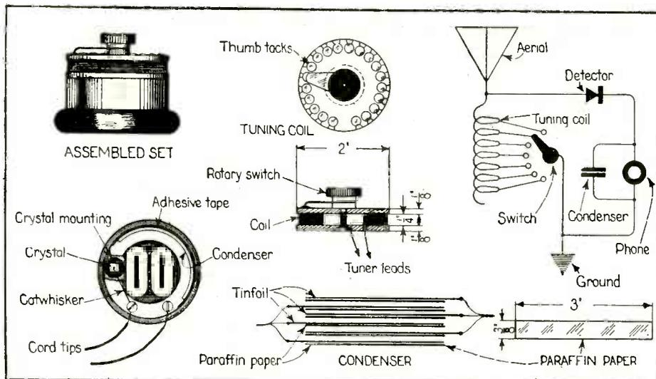
Diagram Above Shows Constructional Details and Wiring Diagram of Pocket Radiophone Receiving Set. All the Parts are Mounted Within or on Watch-Case-Type Receiver Shell.
