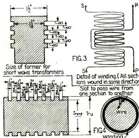
Fig. 3. Constructional Details of the Inter-Tube Transformers Are Given in This Sketch. As May Be Noted, the Primary Winding is Wound in Sections Sandwiched Between Those of the Secondary.
