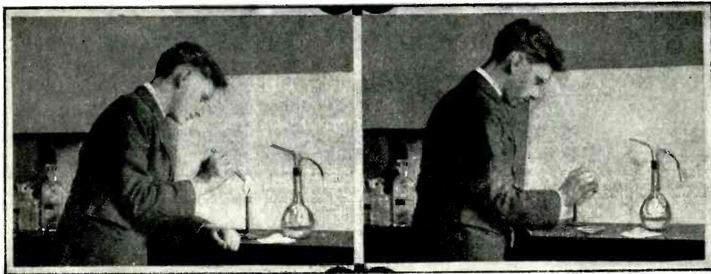
Left—Caution Must Be Exercised Here When Making the Preliminary Tests Where a Substance Is Heated in a Closed Tube. Right—Treating for Chloric Acid by Cautiously Dropping a Bit of the Substance into a Watch Glass Containing 2 C.C. of Concentrated Sulphuric Acid.
