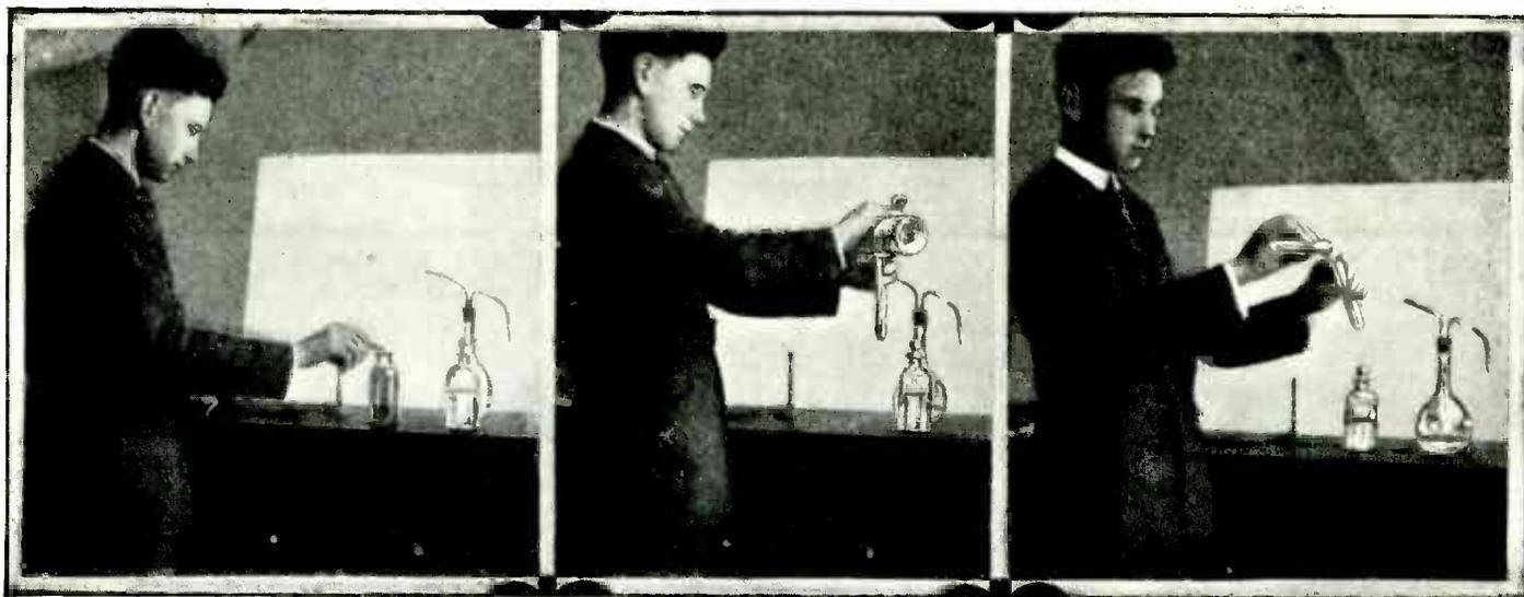
Left—Making the Starch Test for Iodine by Pouring the Iodine Solution into Very Thin Starch Paste and Obtaining a Blue Color. Center—Making the Brown Ring Test for a Nitrate. The Test Is Quite Sensitive and the Ring Clearly Defined. Right—Testing for Iron Salts. All of the Tests Here Shown Are Quite Simple.
