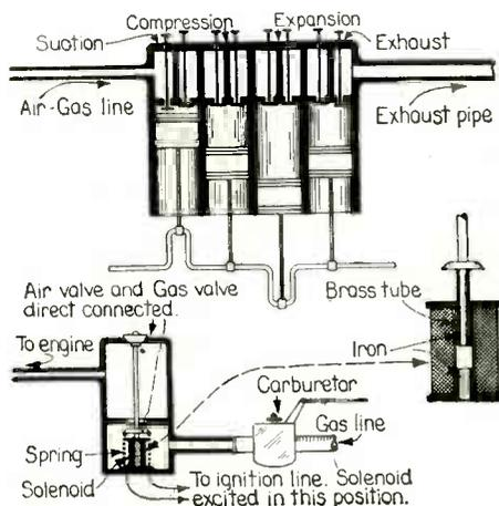
A Magnetically Controlled Fuel Economizer Valve, Which Cuts Off the Gasoline Supply When Coasting Down Hills, etc.
