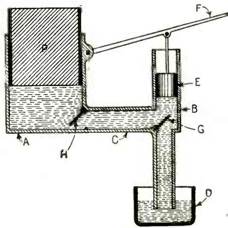
A Simplified Diagram Showing How a Hydraulic Press Operates Is Given Here. A Complete Description Is Given in the Text. If the Cross-Sectional Area of E Is 10 and That of P Is 100, the Piston P Will Move Only One-Tenth as Far as E.
