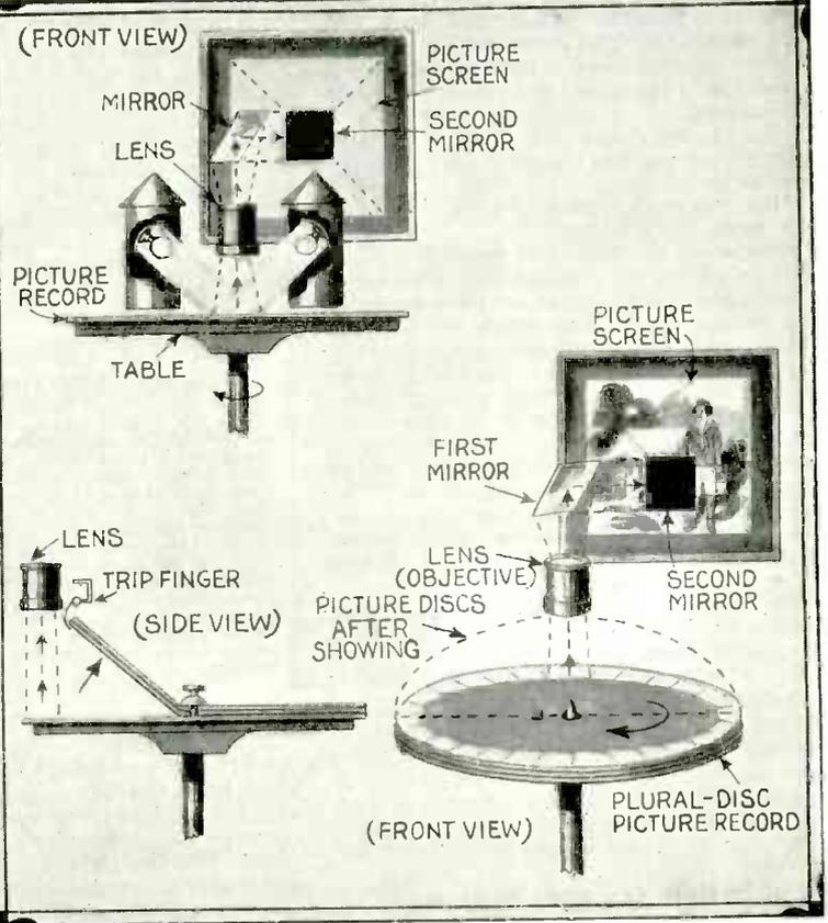
The Newest Movie-Phonograph Is Illustrated Above With Its Inventor, Mr. C. Francis Jenkins, of Washington, D. C. The Diagrams at the Right Show How the Reflected Light From Two Small Lamps Is Caused to Reflect the Image Up Through the Objective Lens or to the First Mirror, Thence on to a Second Mirror and From That on to the Screen, Which Is Placed in the Top of the Phonograph Cabinet Lid. No Celluloid Film Is Used, the Pictures Being Printed on Paper, Any Fire Hazard Thereby Being Obviated.
