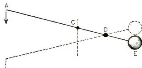
A Fallacy in Levers Is Shown Here. The Idea Is to Balance the Lever AD by the Weight E. So That More Power Will Be Applied to C. When Work Is Performed on A. How This Lever Works and Why the Latter Is Not True, Is Set Forth in the Text.
