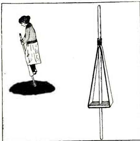
The Popular "Pogo" or Jumping Stick Is Easily Constructed, as Shown in the Illustration Above, the Resilient Step or Foot Rest Being Suspended on a Piece of Old Inner Tube Instead of Springs.
