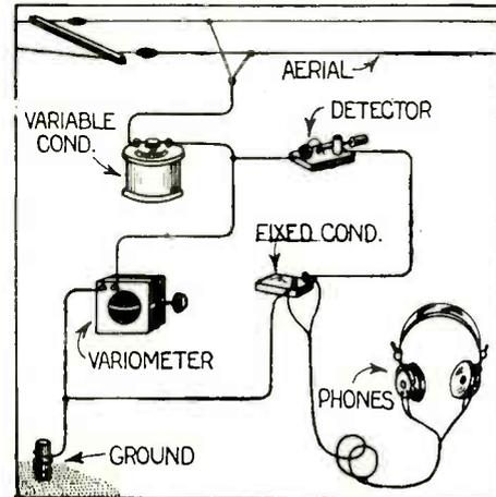
A Simple Crystal Detector Circuit Using a Variometer and a Variable Condenser for Tuning, Is Given Above.
