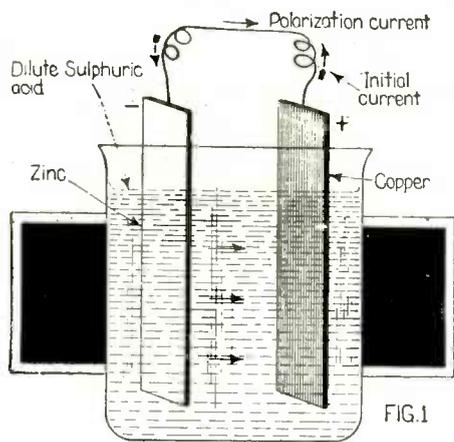
Fig. 1. A Simple Primary Cell. On Connecting the Zinc and Copper Electrodes With a Wire as Shown, a Current Is Generated. Bubbles of Hydrogen Soon Cover the Copper Electrode, However, and the Current Falls to Zero.
