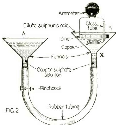
Fig. 2. The Instant Effect of a Depolarizer Can Be Shown by Using the Above Simple Apparatus. As the Current Which the Battery in Funnel B Is Producing, Dies Down Owing to Polarization, Funnel A Is Raised, Thus Bringing the Copper Sulphate Depolarizer into Action. The Current Then Builds Up.
