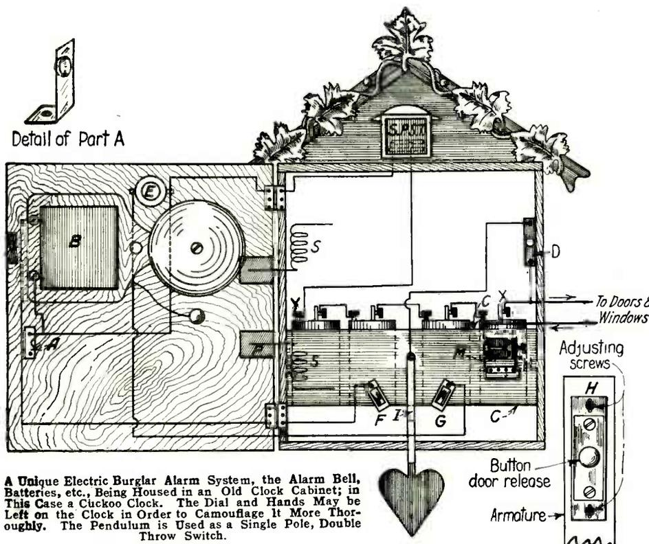
A Unique Electric Burglar Alarm System, the Alarm Bell, Batteries, etc., Being Housed in an Old Clock Cabinet; in This Case a Cuckoo Clock. The Dial and Hands May be Left on the Clock in Order to Camouflage It More Thoroughly. The Pendulum is Used as a Single Pole, Double Throw Switch.
