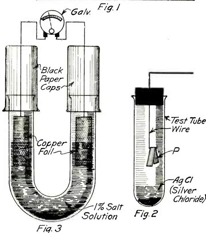
Fig. 1. A shallow Photo-Developing Tray Can Be Used to Show Photochemical Extinction. Fig. 2. Silver Chloride Blackens on Exposure to Light, the Blackening Being Approximately Proportional to the Intensity of the Light. Fig. 3. Using This Simple Cell, Light Produces a Chemical Reaction, and the Chemical Reaction Causes an Electric Current to Be Set Up.
