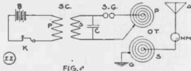
or geissler tube to indicate when maximum radiation occurs, OT, the oscillation transformer, C, high potential condenser, SG, spark gap, and the balance of the instruments as indicated.
