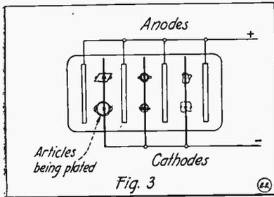
Below is given a table of the usual potentials employed for various kinds of electro-plating. The voltage should be specially adjusted for each case to give the most suitable current, and depends upon the size of the plating tank, the area of the anodes, the strength of the solution, and several other things, and most platers determine the best potential and current for a certain purpose by experiment.
