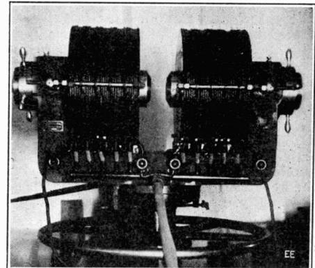
A 40 Kilowatt experimental electro-magnet with water cooled coils.
