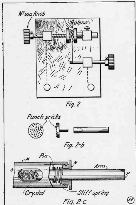
importance than the lightness of the contact. For this purpose a short piece of 36 or 38 gauge copper or phosphor bronze, gold, etc., wire should be fastened at one end, and the other allowed to rest by its own weight on the galena.
