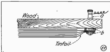
in the drawing where b, b are pieces of brass about  $\frac{1}{4}$ " wide,  $\frac{1}{8}$ " thick and about 2" long. A, is one of the E. I. Co. No. 1,919 rubber binding post. A  $\frac{1}{8}$ " hole is bored in both pieces of brass at the center of same.
