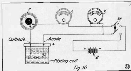
It is advisable to measure the voltage and amperage of the plating, current for any serious work, and the instruments appearing in Fig. 9 are admirably suited to this work. The arrangement of a complete plating
