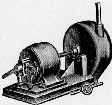
Fig. 11. Water motor direct connected to dynamo. The double sulphate, as given above, is widely used for nickel plating. The chloride may also be employed as a basis for nickel plating, as per the following formula.
