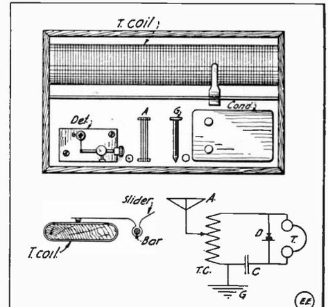
Detectors. For an aerial a 20 foot length of bare copper wire is stretched from a tree limb down to the instruments. Merely sink a nail into the earth for the ground.
