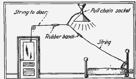
keep from breaking the socket when it is jerked too hard in opening the door.
