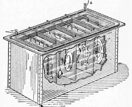
Fig. 5. How Various Articles Are Suspended in Plating Tank
