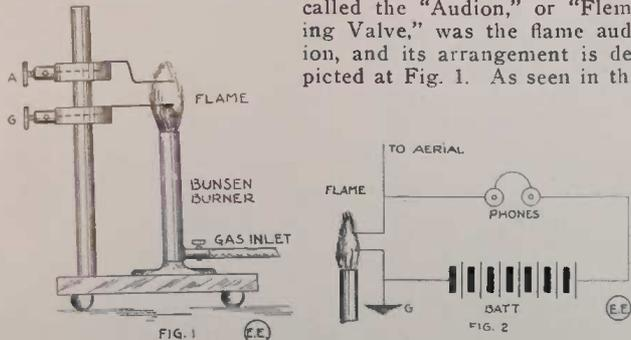
drawing, an ordinary Bunsen gas flame is utilized, and in this flame are placed two conductors or electrodes. It was found that the best form of the flame audion was that involving the use of a Bunsen flame, burning coal gas, and having in its flame two electrodes, as shown; one of them (the lower) being a small platinum trough or cup, and the upper electrode a platinum point.
