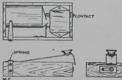
The spring finger makes contact with a key mounted on the box cover. This key, which is made of phosphor bronze, is of the
