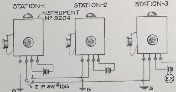
instruments as stated in your question, and, as will be seen, a two-point switch is all that is required at No. 1 instrument, so that by moving the switch lever to No. 2 or No. 3 contact points, No. 1 party can talk to either No. 2 or No. 3, but normally the switch lever is left at No. 2 point, so that No. 2 party can at any time call up No. 1 if desired, and vice versa.
