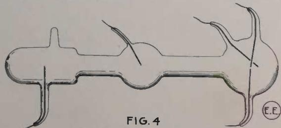
since it is known that at the cathode the great resistance to discharge is situated. In this manner a Hertzian spark too feeble to be visible at a distance can be rendered manifest by its power to start off another discharge from a powerful battery acting on the same mass or rarefied gas.
