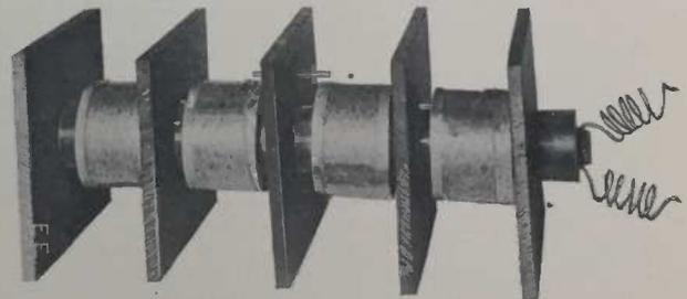
Fig. 3. Stout Pieces of Glass Tubing Lead the Wires from One Secondary to the Next One.
