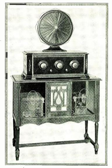
Illustration showing the Inexpensive Five Tube Receiver installed in console
