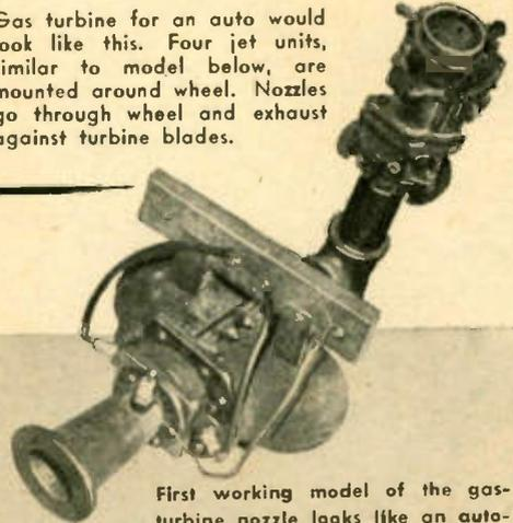
First working model of the gas-turbine nozzle looks like an automobile horn with puffed cheeks.
