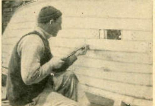
**8** Take care with the planking to get an exact fit, and then bevel the edge for calking. Holes are bored and countersunk deeply, and the screws are put into the butt blacks and frames.
