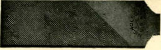
It's the kind of perfect-fit finish that usually results when human skill and *The right file for the job* get together. A Nicholson Long Angle Lathe File is shown removing the last few thousandths inch from a shaft. The same file will do the final smooth-finishing.
