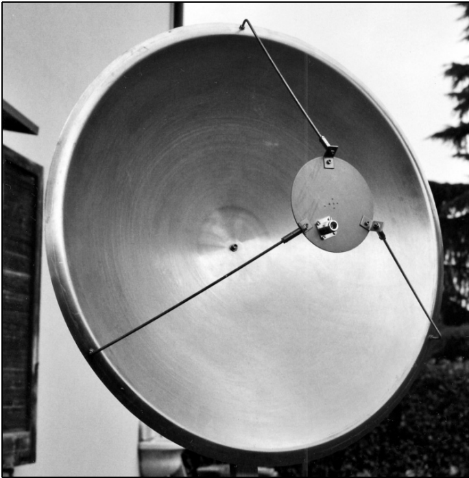
Fig 9: The complete 60cm dish antenna with the feeder and the support arm.
