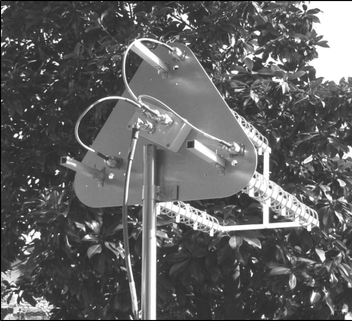
Fig 3: A 3 x 16.7 turn TriHelix antenna.
