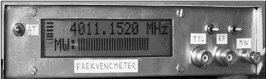
Fig 17: The counter in the microwave mode with a gate time of 640ms corresponding to a resolution of 100Hz.
