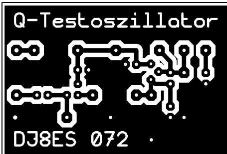
Fig 3: PCB layout for the crystal test oscillator.
