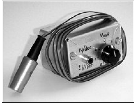
Fig 11: Picture of the LOG102 amplifier front panel.
