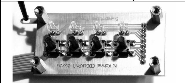
Fig 15: PCB layout for electronic sweep time keys.
