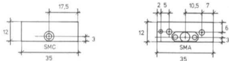
Fig.6.5 End plate and Connector details DL1RQ 661
