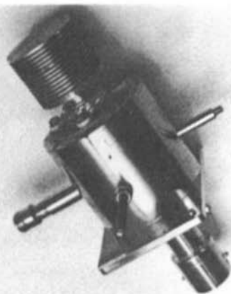
Fig.4 A 13cm PA with a modified 2C39BA
