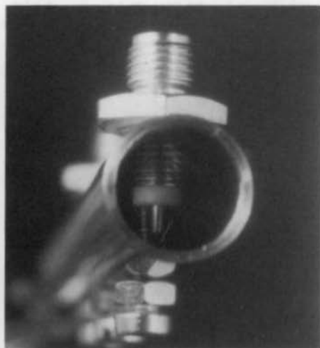
Fig. 3: Coupling by means of the SMA-socket's spigot
