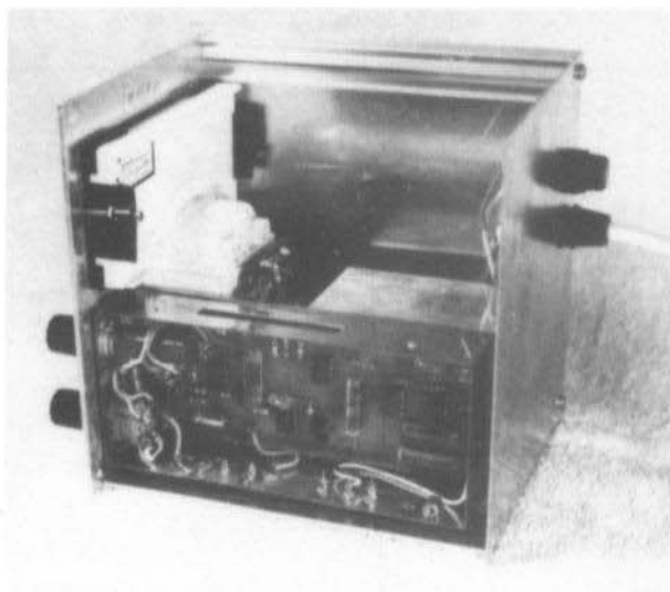
Fig. 23: In the completed instrument, the cover has been removed to show the board. The small power supply unit is located behind it in a second tin-plate box
