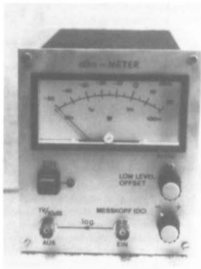
Fig. 1: A dBm-meter with a 70 dB indicator dynamic range (scaled for low-barrier diodes)
