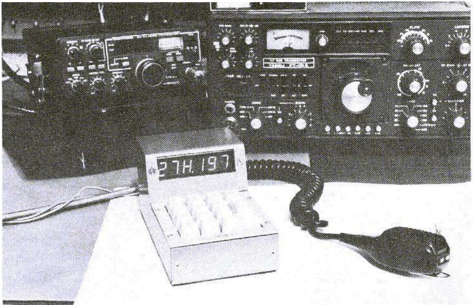
Fig. 2: Author's prototype control unit showing 27° elevation, manual operation (H), and 197° azimuth
