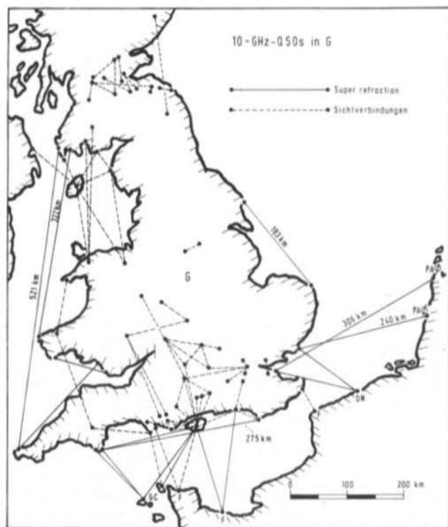
Fig. 1: Some of the paths worked on 10 GHz by UK amateurs. The 521 km contact probably is the world record.
