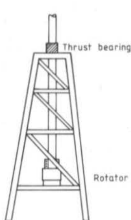
Fig. 3: Mounting of a rotator in a tower
