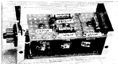
Completed bandpass filter assembled in a Minibox, less cover. Interconnections between the 2490-pf. and 0.0215- \mu f. capacitors, mounted on the top side of the perfboard, can be seen in this view.
