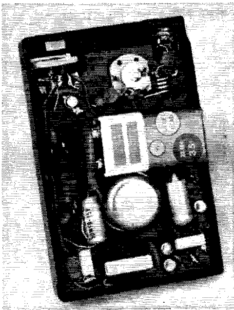
Fig. 2—Inside view of the pocket receiver. The detector circuit is at the top of the unit. Audio gain control R_3 is at the upper left. Transformer T_1 is shown at the lower left corner of the circuit board, just below the 2.5-mh. r.f. choke, RFC_2 . The audio-amplifier circuit is visible at the lower right.
