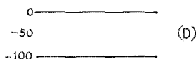
Waveform D Measured between Grid No. 1 (pin 2) of the vidicon and chassis, with beam control fully counterclockwise.
