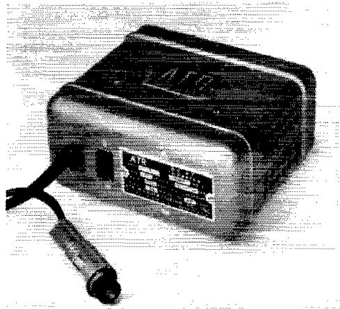
The ATR 50-watt inverter. The plug in the foreground inserts into the car cigarette lighter, for d.c. power pick-up. Output, 117 volts, 60 cycles, appears at the receptacle just to the left of the name plate.
