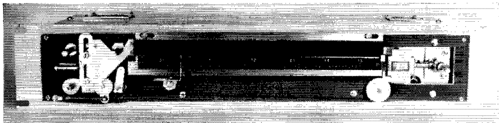
Front panel of the 3-4-Mc. tuner unit with cover removed. The digital counter at the right is driven from the tuning shaft by means of small bevel gears. The turning shaft has a ball bearing at each end, and the knob has a built-in friction drive to prevent damage to the gears if the shaft is turned to the end of travel. The mechanism at the left shifts a masking strip that hides the frequency scale not in use. Another shaft and arm shifts the position of the frequency scale to correct the calibration as needed.
