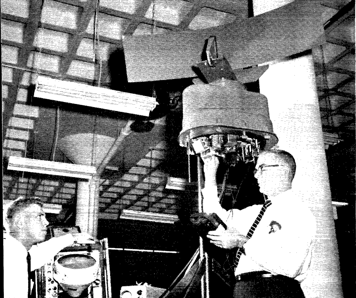
STEPHEN HERZOG (left), K5RMA, and George Mayo, K1LYE, check out marine radar equipment at a Raytheon Electronic Services Division service center in Boston, Mass.
