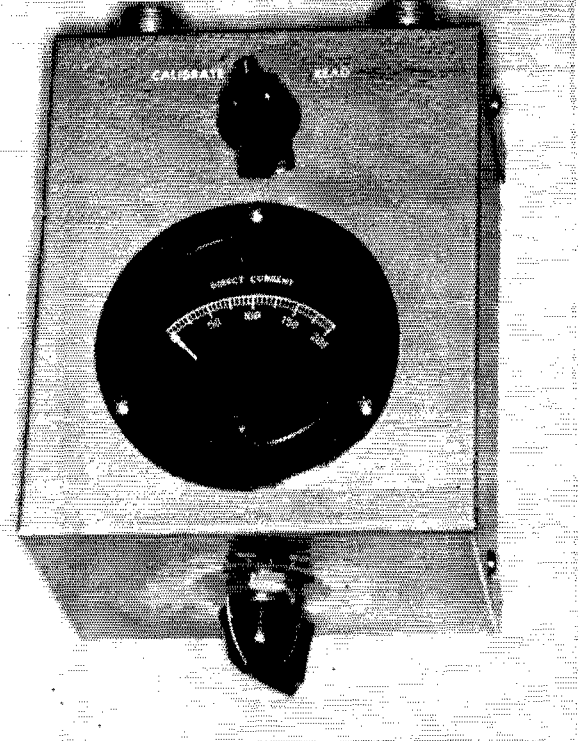
This s.w.r. indicator features simple construction using ordinary coax cable. The forward-reflected switch—labeled "Calibrate" and "Read"—is at the top. The control below the meter is the sensitivity control.
