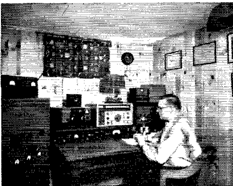
NNJ Official Bulletin Station W2VCZ rolled up the January CD Party's leading phone score at this well-appointed operating position. Gear includes a kw. final and modulator, Ranger, NC300, Viking I and v.f.o. These are intermittently tied to 10-11 and 15-meter rotaries, and to fixed arrays on 40 and 80.
