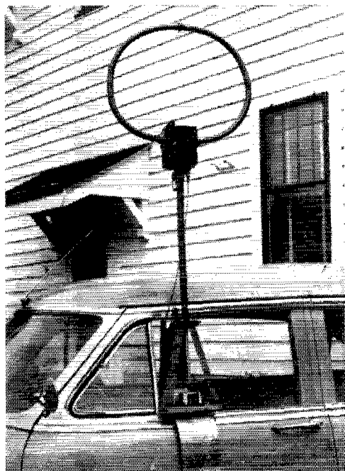
W8YPT's 10-meter d.f. loop antenna. The sense antenna is braced against, but insulated from the loop with rubber tape.
