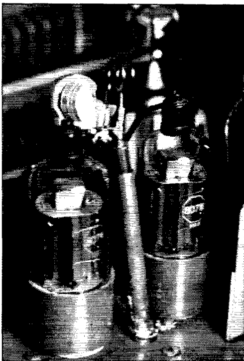
Exciter stage showing copper tube mounted between 807s with insulated lead coming up through the center. Also installed is a plate trap adjusted to Channel 4.
