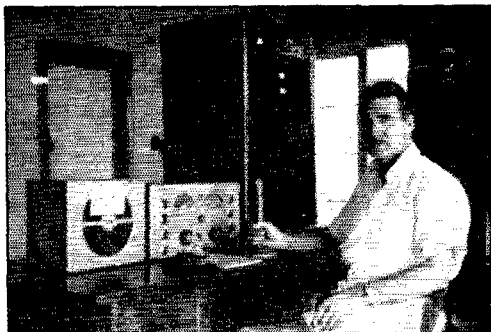
ZK2AA is one of the choicer bits of Pacific DX. Operator Bill Scarborough uses 30 watts to a 2E26, modulated by 6L6s. An NC-183 is the receiver and the various antennae include a long wire on 14 Mc., a 3-element beam for 10, and a 6-meter 4-element rotary.
