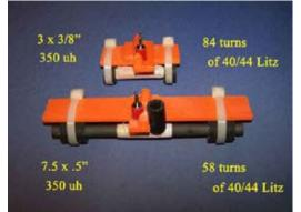
leads were soldered to a Radio Shack 1/8" phone plug, which was glued inside the perpendicular 10mm hole in the frame. No provision was made to avoid loopstick rotation in this simple design, which was not intended to be a final DXing antenna.
