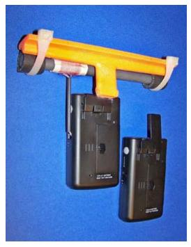
ably use a Velcro mounting system for the DT-200VX, like that described by John Bryant in the E100 Slider Loopstick article (currently posted on , in the Ultralight Radio File section). John has also published subsequent articles describing various ways of mounting the Slider loopstick, which would also apply for this DT-200VX Slider loopstick model in a plywood frame system..
