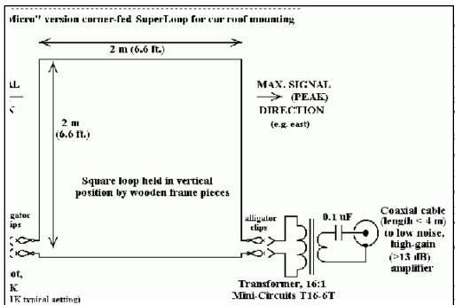
Because of the small dimensions of the antenna, you definitely need low-noise high-gain amplification. A single RPA-1, at about 14 dB of gain, is borderline. At night at the seashore with a band full of big fat TA, Latin American, and domestic signals, it was OK. I am thinking of trying out higher gain amplifiers for situations where more signal output is required: daytime DX, inland DX, auroral DX, post-dawn TP's in western North America, etc.
