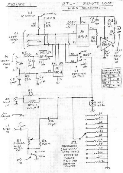
5. Install jacks, pots, and switches. Solder inductors onto S1 per Figure 1 and Tables 2 & 3.
