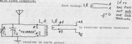
N.B.: On some flat loopsticks "2" and "3" are connected together, if so make sure "2" and "3" are on the grounded side and "1" and "4" are on the "hot" side of the circuit.
