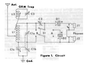
The main tuning circuit consists of a low-loss, high-Q basketweave coil (L1) in parallel with one section (Cla) of a three-gang variable capacitor (Cl). The antenna taps in near the ground side of L1 (autotransformer arrangement) for best loading. The remaining two sections of Cl (Clb, Clc) provide capacitive coupling to ground. Variable ground coupling increases selectivity at the high end and boosts sensitivity at the low end, producing optimum response over the entire tuning range.
