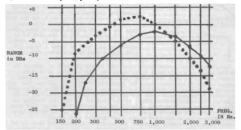
This graph represents the frequency response obtained in my measurements. The dotted line is the coil as wound by the instructions given in this article. You'll note response is good between 200 and 2,000 Hz, with with most of the audio between 300 and 1,000Hz. In reality this causes tapes of music and such to sound rather "bassy".
