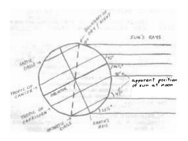
Figure 4-1: Illustration of the Variations in the Sun's Incident Angle Corresponding to Latitude,
