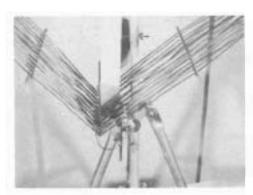
1. Capacitor mounting plate, tripod mount, front view.
