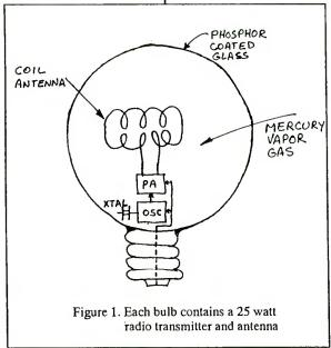
light equivalent to a 100 watt incandescent lamp, the power amplifier drives the antenna with 25 watts of RF at 13.56 MHz. The RF excites the molecules of a mercury vapor gas which in turn emit ultra-violet radiation. This radiation is intercepted by the phosphor
