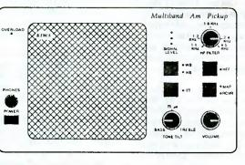
receivers). It connects to the IF stage either through the receiver's IF output jack if it has one. or via microclips to the IF output point on the circuit board. You do not have to modify your receiver to use this, just connect it up.
