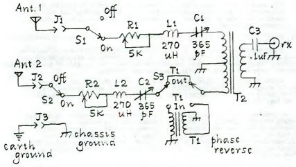
Tl is a phase-reversing toriodal transformer consisting of a 25 turn bifilar winding evenly spaced, occupying 1/2 of a Miller F-87-1 or Amidon FT-82-77 core. (FT-82-61 for tropical bands)
