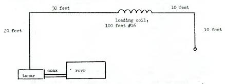
This antenna can also be used outdoors if the loading coil is weatherproofed.
