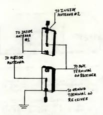
A NOVEL ANTENNA SWITCHING ARRANGEMENT
