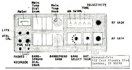
One can see by the illustration above that there are enough controls for adequate DXing functions, including the ever-useful antenna trim. Frequency readings easily within 2-3 KHz, sometimes 1 KHz at low fqy.
