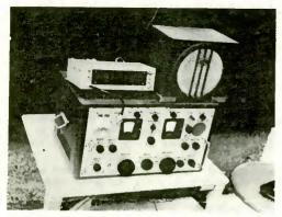
receiver is tuned, to within a nominal range of 100 Hz. This is not the ordinary frequency counter one sees advertised in ham radio magazines, but is one incorporating a pre-programmed offset to allow for the difference between the receiver's local oscillator signal (which drives the counter) and the received signal's frequency. This of course is the receiver's IF freq.
