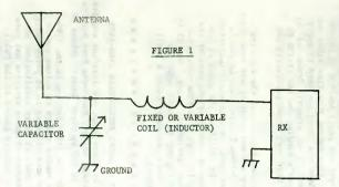
An L network as shown above will not match an antenna to a receiver under all cases of mismatch but will under most cases. The L network can be made to match in all cases by purting the variable capacitor on a switch so it can be switched to the antenna side or the receiver side of the coil as shown below in figure 2.
