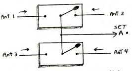
Two Leviton # 9914 single-knife switches connecting four longwires.
